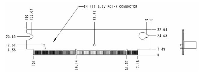
Figure 42. 1U Low-Profile PCI-X Riser Card Mechanical Drawing
