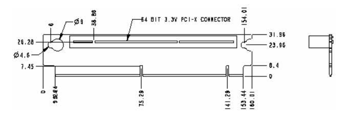
Figure 40. 1U Full-Height PCI-X Riser Card Mechanical Drawing
