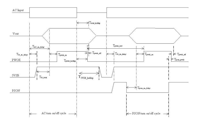
Figure 14. Turn On/Off Timing (Power Supply Signals)
