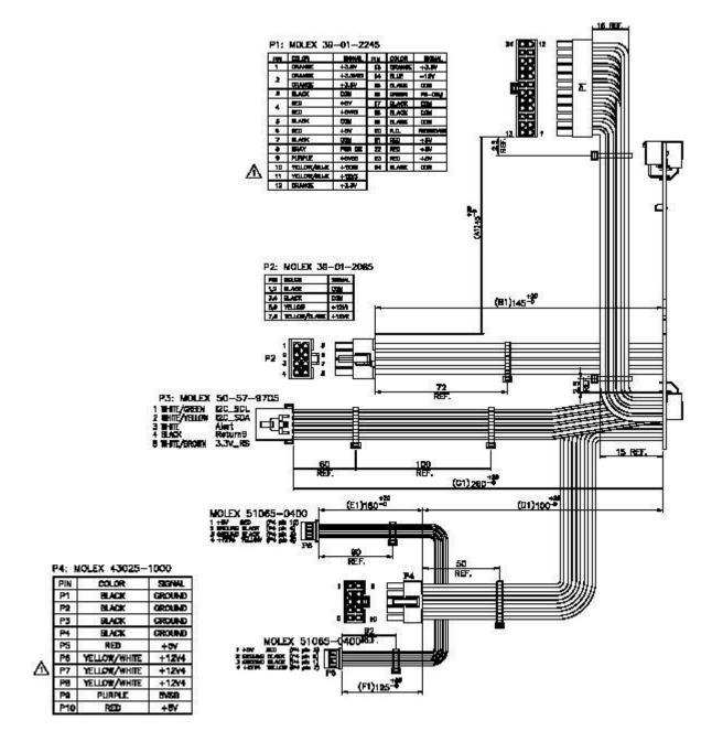
Figure 12. Power Distribution Board Harness Detail
