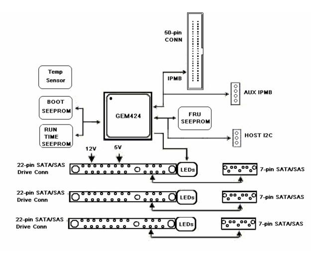
Figure 33. SATA/SAS Backplane Functional Block Diagram
