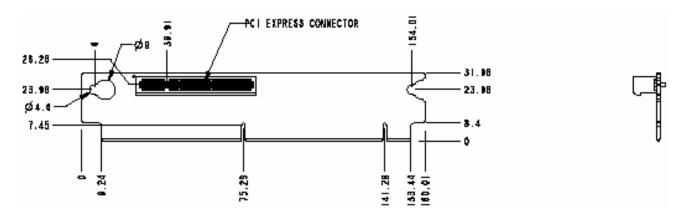
Figure 41. 1U Full-Height PCI-Express Riser Card Mechanical Drawing
