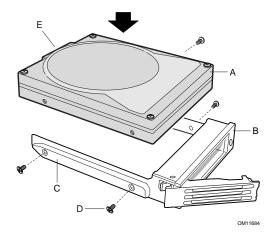
Figure 25. Hard Drive Tray Assembly
