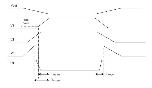
Figure 13. Output Voltage Timing
