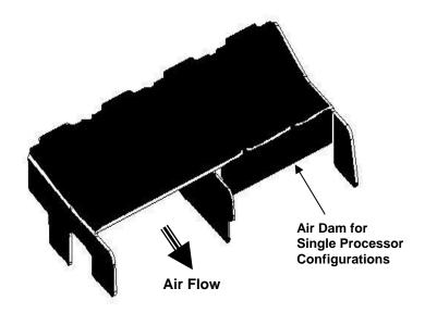
Figure 19. CPU Air Duct
