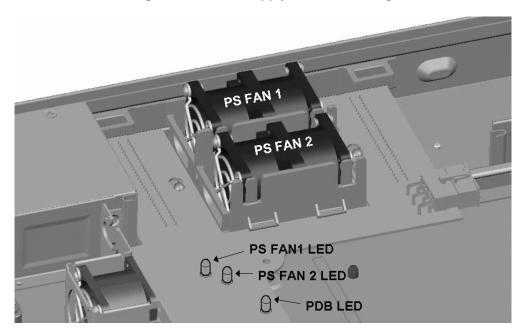
Figure 17. Power Supply Fan Numbering
