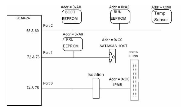
Figure 34. Intel® Server Chassis SR1450 1U SATA/SAS HSBP I<sup>2</sup>C Bus Connection Diagram
