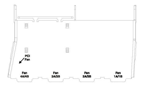
Figure 20. CPU Air Duct Fan Numbering
