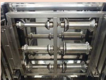
Cables/Wires winding accessory for 'Cold bend' testing
