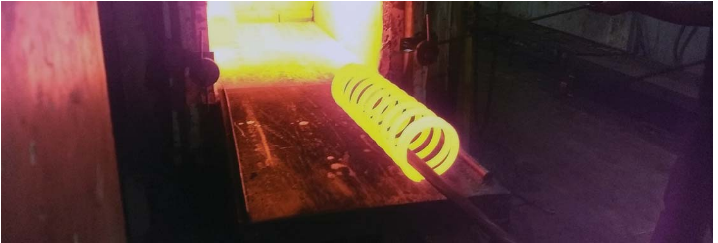
Heat Treatment of Coil Springs
