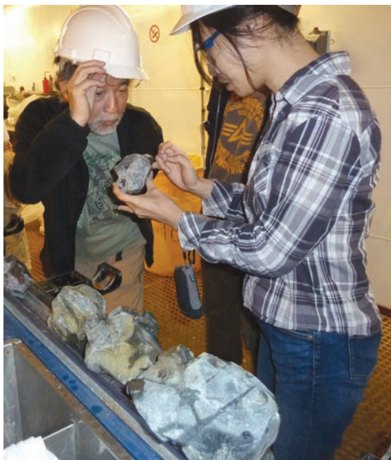
Figure 4: Granoblastic dike samples were recovered in abundance by fishing tools during successive hole remediation operations. Sumiyo Miyashita and Yoshiko Adashi, from Niigata University, examine unusually large rock samples from Hole 1256D.
