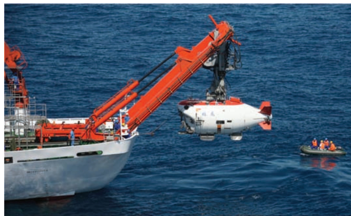
Figure 1: Chinese Dragon manned submersible during a test dive in the East Pacific.
