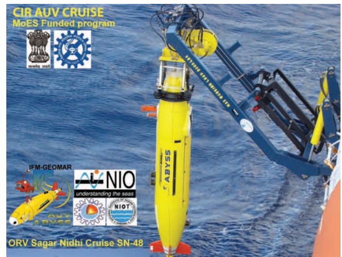
Figure 1: Launching of AUV ABYSS from the Indian research vessel R/V Sagar Nidhi .
