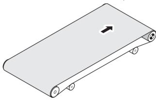
Fig.: Non-reversible conveyor with head drive
