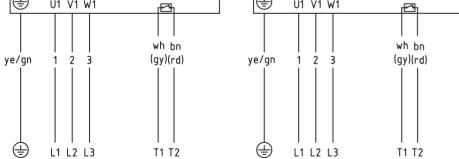
Fig.: 3-phase operation, 4+2 lead cable, winding for 1 voltage, delta or star connection (internally connected)
