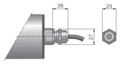
Fig.: Straight connector, brass/nickel or stainless steel
