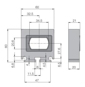
Fig.: Anti-vibration Brackets
