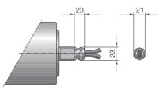
Fig.: Straight connector / Feedback device, brass/nickel
