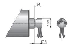
Fig.: Elbow connector, stainless steel
