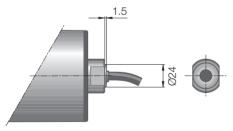
Fig.: Straight cable outlet, PU shaft plug
