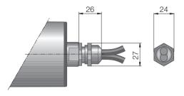
Fig.: Straight connector / Feedback device, brass/nickel or stainless steel
