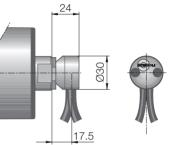
Fig.: Elbow connector / Feedback device,
