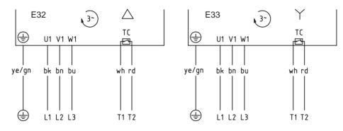
Fig.: 3-phase operation, 6 lead cable, winding for 1 voltage, delta or star connection (internally connected)
