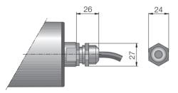
Fig.: Straight connector, brass/nickel or stainless steel
