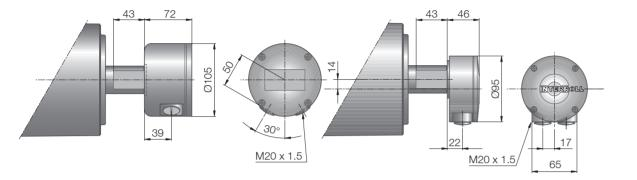
Fig.: Terminal box, technopolymer
