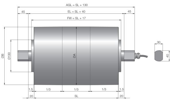
Fig.: Drum motor with straight connector
