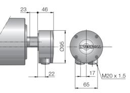
Fig.: Terminal box, aluminium
