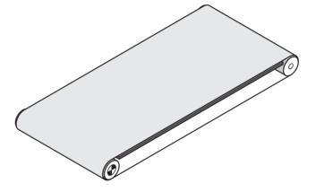
Fig.: Slide bed conveyor
