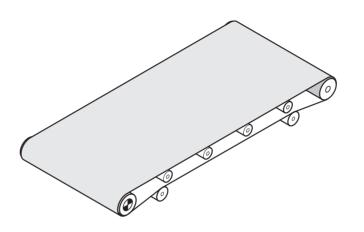
Fig.: Roller bed conveyor
