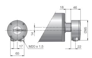
Fig.: Terminal box, aluminium
