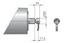
Fig.: Elbow connector, technopolymer
