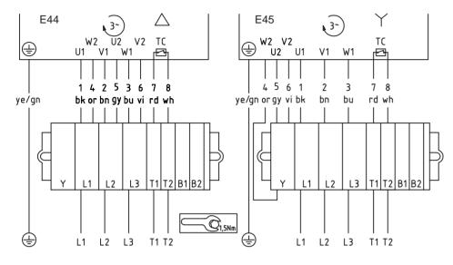
Fig.: 3-phase operation, 9 lead cable, winding for 2 voltages, delta or star connection Note: The screws of the terminal box lid have to be tightened with a torque of 1.5 Nm. Delta connection: Low voltage Star connection: High voltage
