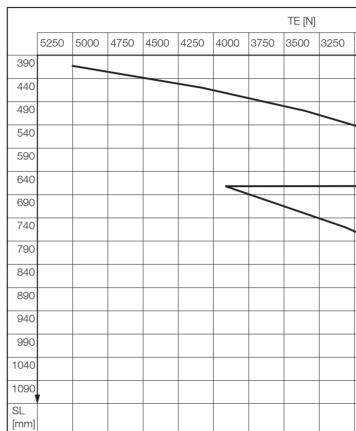
Note: To get the right value of the maximum allowed belt tension, first find the maximum allowed TE value for the drum motor RPM. For motors with SL > 400 mm, check if the maximum allowed TE value for the SL is lower. In this case, use the lower value as maximum allowed TE value. TE Belt Tension n<sub>A</sub> SL nell
