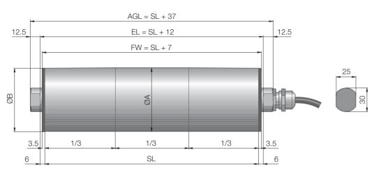
Fig.: Drum motor with straight connector
