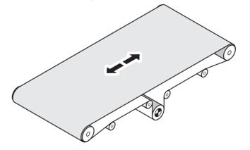
Fig.: Long belt conveyor with centre drive
