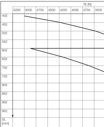
**Note:** To get the right value of the maximum allowed belt tension, first find the maximum allowed TE value for the drum motor RPM. For motors with SL > 402 mm,check if the maximum allowed TE value for the SL is lower. In this case, use the lower value as maximum allowed TE value.
