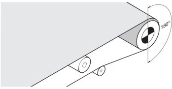
Fig.: Minimum belt wrap angle for friction drive belt conveyors
