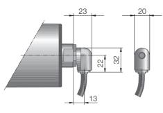
Fig.: Elbow connector, technopolymer
