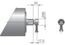
Fig.: Elbow connector / Feedback device,
