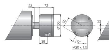
Fig.: Terminal box, technopolymer
