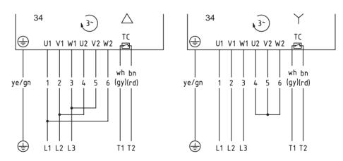
Fig.: 3-phase operation, 7+2 lead cable, winding for 2 voltages, delta or star connection
