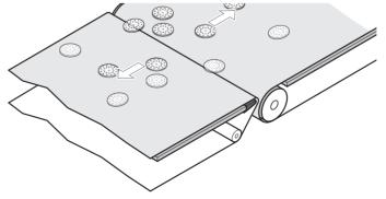
Fig.: Knife-edge conveyor
