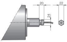
Fig.: Straight connector, stainless steel
