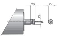
Fig.: Straight connector, stainless steel
