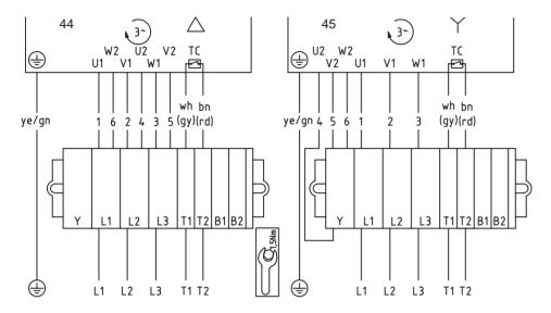
Fig.: 3-phase operation, winding for 2 voltages, delta or star connection Note: The screws of the terminal box lid have to be tightened with a torque of 1.5 Nm.
