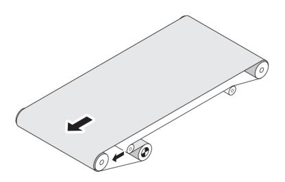
Fig.: Centre drive for long belt conveyor with increased belt wrap
