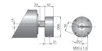
Fig.: Elbow connector / Feedback device, stainless steel
