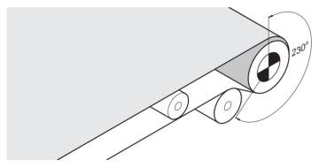
Fig.: Increased belt wrap angle for friction drive belt conveyors
