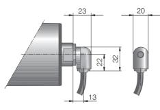
Fig.: Elbow connector, technopolymer
