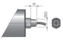
Fig: Straight hygienic connector, IP69k stainless steel
