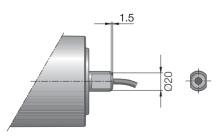
Fig.: Straight cable outlet, PU shaft plug
