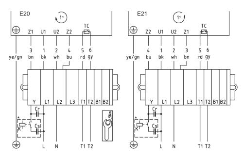
Fig.: 1-phase operation, 7 lead cable Note: \*Further information for starting relay, see p 204.
