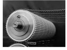
Plastic modular belts, solid homogeneous belts, steel mesh or wire belts are positively driven with no tension. Because the belt has very little direct contact with the drum shell, heat dissipation is less effective and therefore the drum motor should be used in conjunction with a frequency inverter optimised for this application. Alternatively a motor for applications with positive drive belts or no belts, or a synchronous drum motor can be used.
