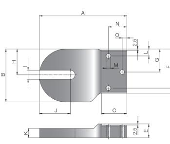
Fig.: Right-hand side bracket (A) for drum motor with elbow connector, straight connector or terminal box
