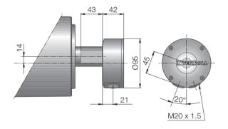
Fig.: Terminal box, stainless steel
