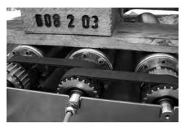
For applications without a conveyor belt or narrow belt, covering less than 70 % of the drum motor face width, heat from the motor cannot be dissipated via the belt contact and therefore asynchronous drum motors must be optimised for applications with positive drive belts or no belts. This can also be done with a frequency inverter. Alternatively a synchronous drum motor can be used.
