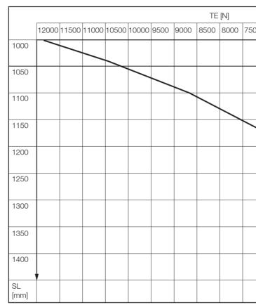
**Note:** To get the right value of the maximum allowed belt tension, first find the maximum allowed TE value for the drum motor RPM. For motors with SL > 1,000 mm,check if the maximum allowed TE value for the SL is lower. In this case, use the lower value as maximum allowed TE value.
