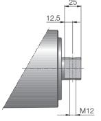
Fig.: Shaft, cross-drilled and threaded
