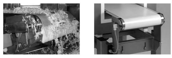
Friction drive belts use the friction between the drum motor shell and belt to drive the belt. The drum motor is normally crowned to prevent belt wander. The belt must be tensioned in order to transmit the torque from the drum motor. The top surface of the belt can be flat, plain or have a ribbed, grooved or diamond pattern.
