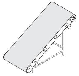
Fig.: Inclined conveyor
