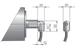
Fig.: Elbow connector, technopolymer
