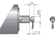
Fig.: Elbow connector, stainless steel
