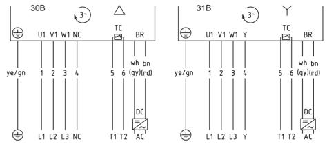
Fig.: 3-phase operation, 7+2 lead cable, winding for 1 voltage, delta or star connection
