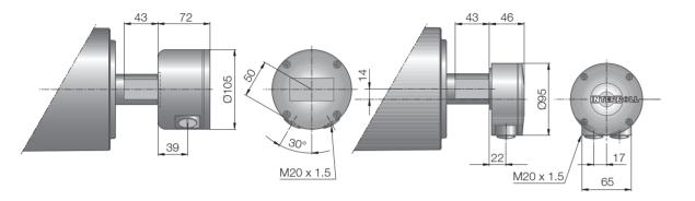
Fig.: Terminal box, technopolymer
