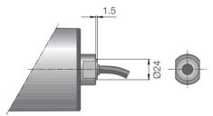
Fig.: Straight cable outlet, PU shaft plug
