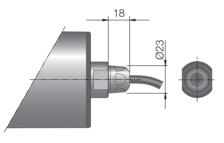
Fig: Straight hygienic connector, IP69k stainless steel
