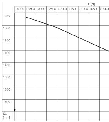
**Note:** To get the right value of the maximum allowed belt tension, first find the maximum allowed TE value for the drum motor RPM. For motors with SL > 1,250 mm,check if the maximum allowed TE value for the SL is lower. In this case, use the lower value as maximum allowed TE value.
