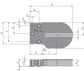
Fig.: Left-hand side bracket (B) for drum motor and idler pulley
