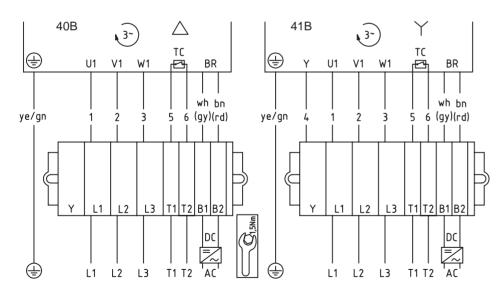
Fig.: 3-phase operation, winding for 1 voltage, delta or star connection, with brake (internally connected)
