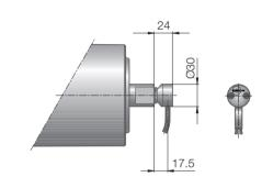
Fig.: Elbow connector, technopolymer
