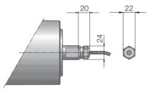
Fig.: Straight connector, stainless steel
