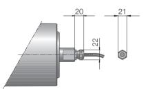
Fig.: Straight connector, brass/nickel
