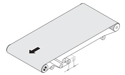
Fig.: Optional design for non-reversible long conveyor with centre take-up
