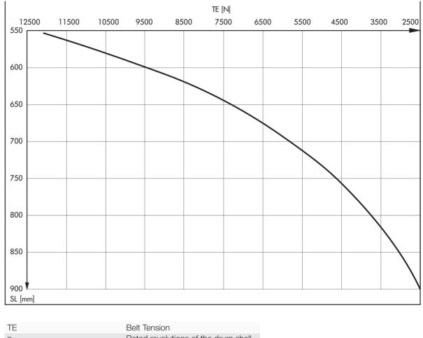
Rated revolutions of the drum shell n\_ SL Shell length
