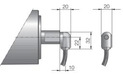
Fig.: Elbow connector, technopolymer
