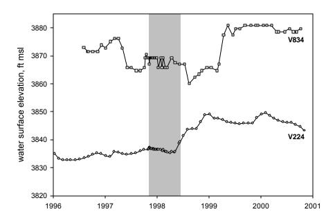
Figure 7. Deep wells near 375W. Gray indicates when 375W was on.
