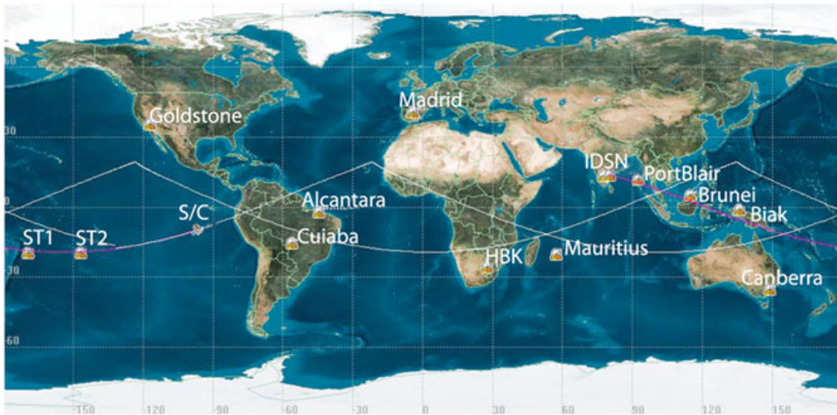
Figure 3.3-5. Network off Ground Stations used in MOM communication
