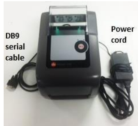
Figure 9 Datamax printer with pre-installed cable
