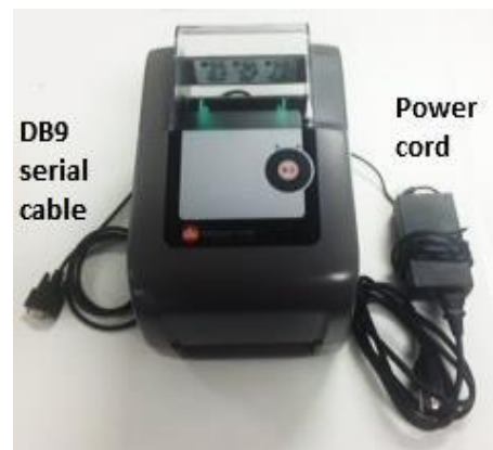
Figure 5 Datamax printer with pre-installed cable
