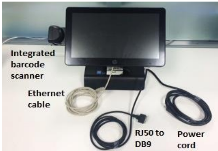
Figure 2 HP RP2 with pre-installed cables
