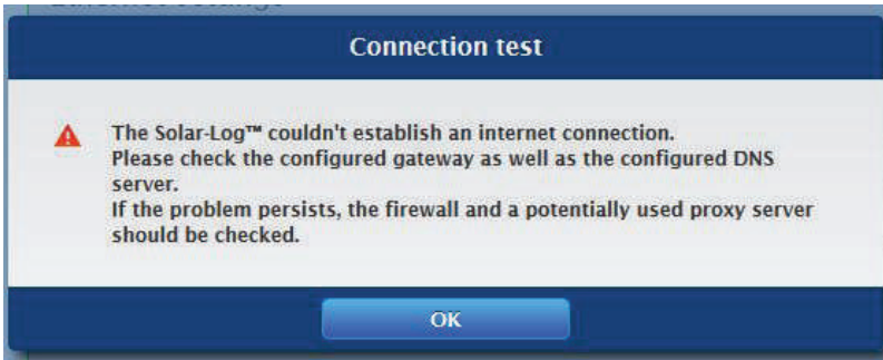
Fig.: Example of an unsuccessful connection test
