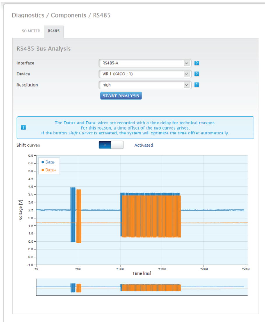
Fig.: RS485 bus analysis with Janitza as an example (with installation mode active)
