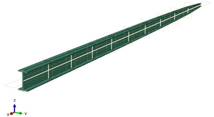
Figure 4.3: Mesh model of Tapered Spar Beam
