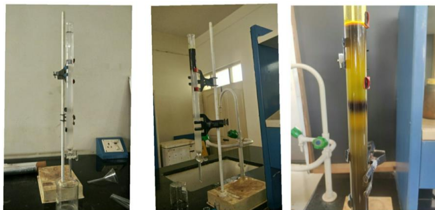
Fig 7: Separation of Bands using Column Chromatography
