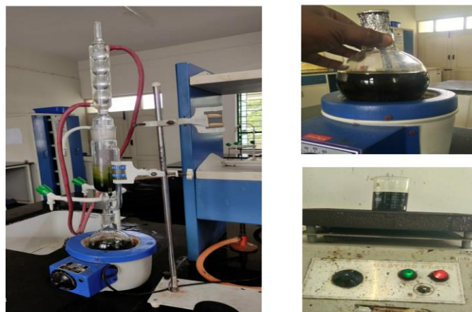
Fig 6: Soxhlet apparatus for extraction and concentrating extracted product
