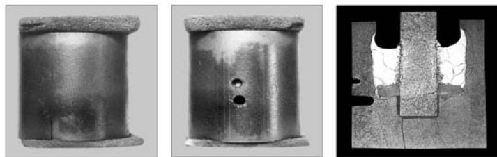
Fig. 2: RIAR 1 est 2 on simultaneous dissolution of \text{UO}_2 and \text{ZrO}_2 ( 2200^{\circ}\text{C} , 200 s).
