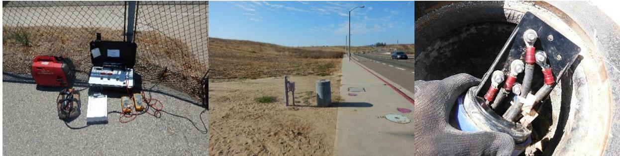
*“Attenuation” Continuity Test Method Setup*
