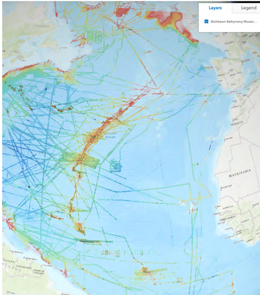
Figure 4.2. Colour shaded relief visualization of gridded multibeam bathymetric data from surveys archived at NOAA's National Centers for Environmental Information (NCEI). https://noaa.maps.arcgis.com/home/item.html?id=6b16e66ffd3740b5820875ad0af25042 accessed 22 August 2019
