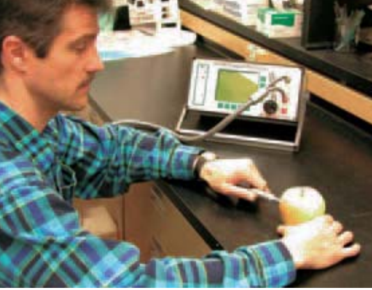
Figure 4. Example of a typical manually-operated chlorophyll fluorescence system. Chlorophyll fluorescence measurement using this type of system is expensive, manual, time-consuming and incapable of sampling large areas of a fruit or vegetable.
