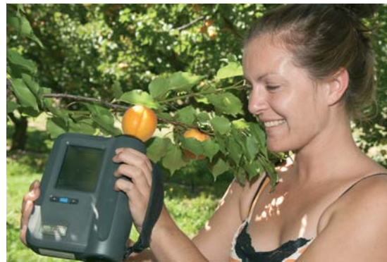
■ Using a portable near infrared spectrophotometer to estimate soluble solids concentration of apricot fruit in an orchard. Photo courtesy of Robert Lamberts, The New Zealand Institute for Plant & Food Research Limited.
