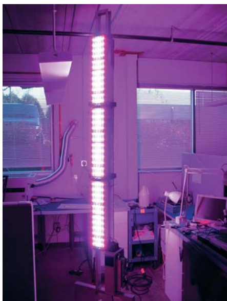
Figure 4. A newly constructed ORBITEC light tower to provide intra-canopy lighting of tall greenhouse crops in two directions within rows. Two-foot-long panels of red and blue LEDs can be switched on or off individually.
