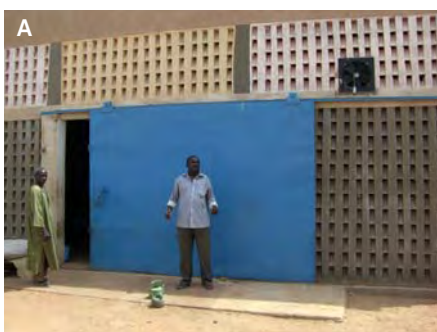
Figure 2. A. Massive onion store building in Gaya with aeration holes. Expensive and unsuitable. B. Metal cages for onion storage in Gaya. Not enough aeration.
