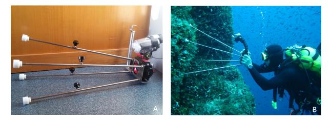
Figure 3.2 – Example of a stainless steel frame with adjustable surface and spacer (A) and its use in the field (B)
