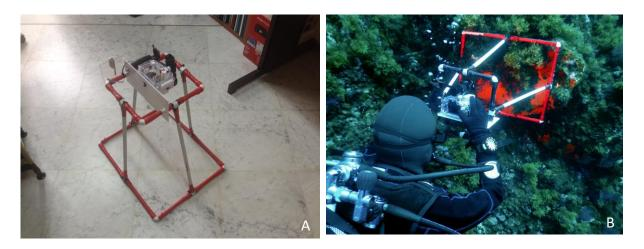
Figure 3.1 – Example of a pvc frame with fixed surface and spacer (A) and its use in the field (B)
