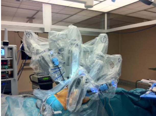
Figure 5. Articulating arms of the da Vinci Si® robotic surgery system (The robot)
