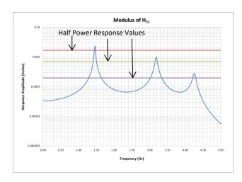
Figure 5 – Modulus Response of  $H(\omega)_{31}$
