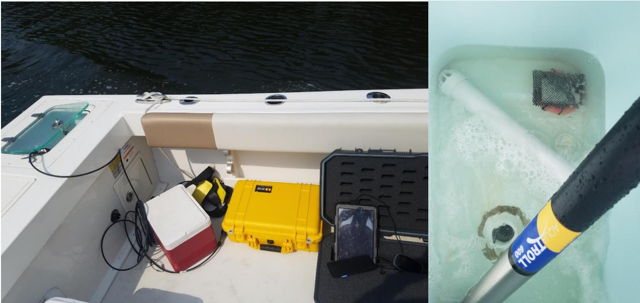
Figure 2: Integrated livewell application for continuous monitoring and toxin tracking during VDH sampling cruise.
