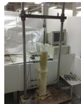
Figure 28. Stress-dependent 1D soil column (Ng & Leung 2011)
