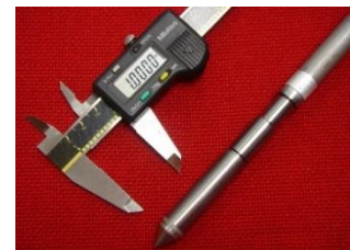
Figure 56. Miniature cone penetrometer for geotechnical centrifuge model testing
