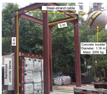
Figure 66. Pendulum impact facility (Ng et al. 2016a)
