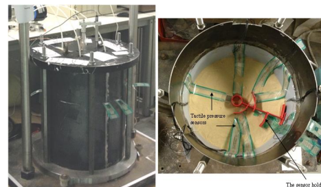
Figure 48. Pressure chamber with advanced sensing devices for model pile test (Zhang & Wang 2015)
