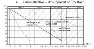
Figure 1. Delimitation of grain size distribution areas from the point of view of soil-stabilization with lime (Kézdi, 1967., Szendefy, 2008.)
