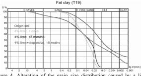
Figure 4. Alteration of the grain size distribution caused by a lime treatment of medium clay soil
