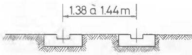
Fig. 92 - Simplified Greek road with two grooves cut into the stone, for guiding the carriages.
