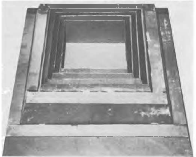
Fig. 40 - Model of the arrangement of blocks used in a step pyramid - L. Kérisel.
