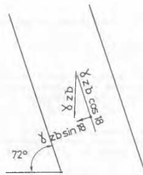
Fig. 133 - Arching theory for sloping walls.
