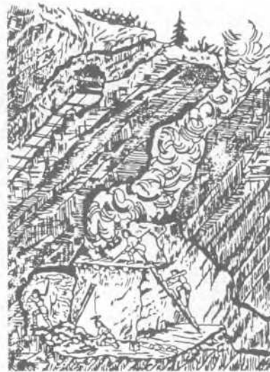
Fig. 108 - Reconstruction of a fire in a copper mine in Mitterberg, Tirol, in order to break up the rock. (1600 to 800 B.C.).
