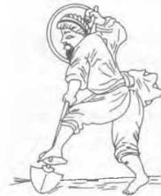
Fig. 63 - Spade with foot support (after Dumas).
