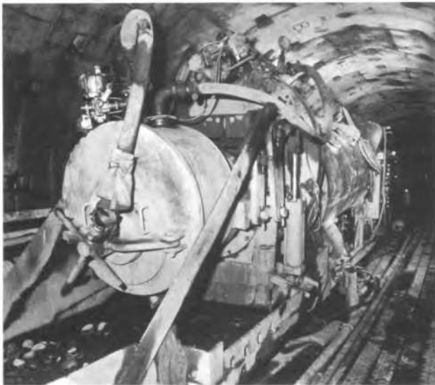
Fig. 6 Apparatus to remove gravel, part of a slurry mole (courtesy of Tekken Construction Co.)
