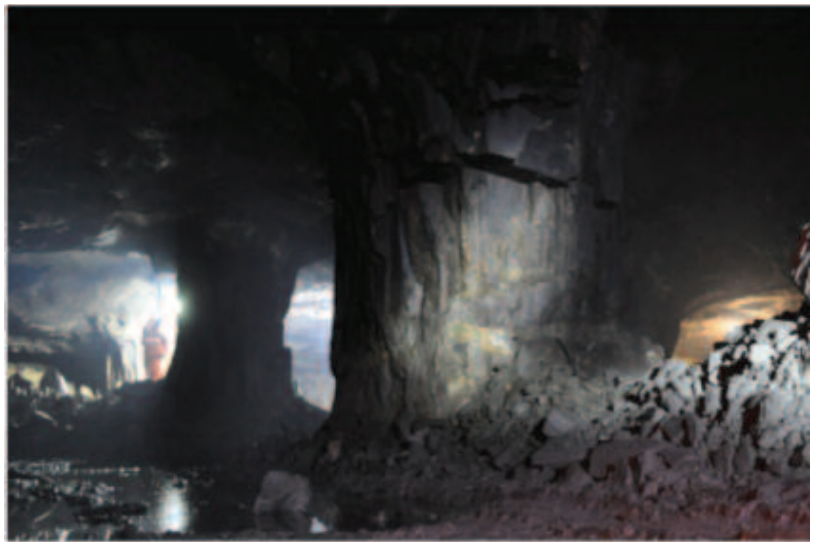
Figure 15 (above): Narrow-vein open stoping, using small pillars as support, San Finx, Spain.
