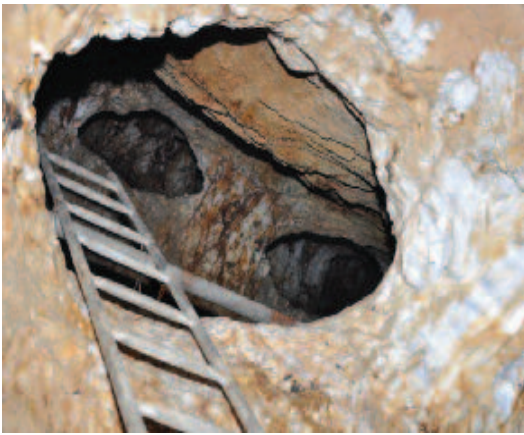
Figure 15 (above): Narrow-vein open stoping, using small pillars as support, San Finx, Spain.
