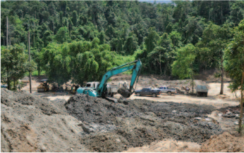
Figure 52: Tailings Retreatment: Rehandling and homogenisation of tailings at the historic Sritorranee mine near Chiang Mai ahead of transport to the flotation plant at Lampang Mineral and Metal (Thailand) Ltd.
