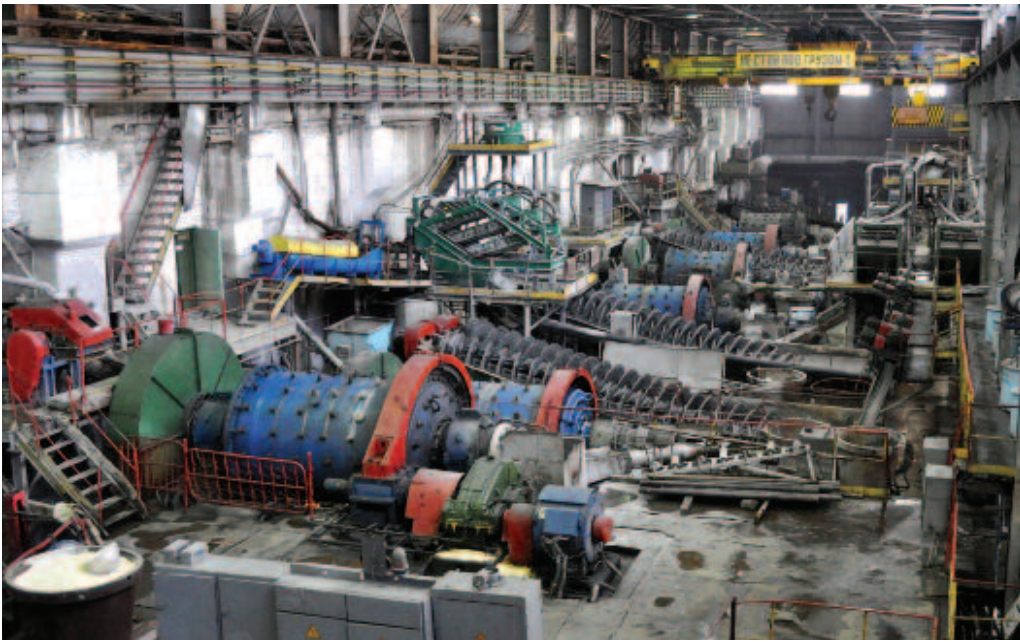
Figure 29 (left): Milling: Staged rod and ball mills and spiral classifiers at the Vostok-II mine, Far-East Russia.
