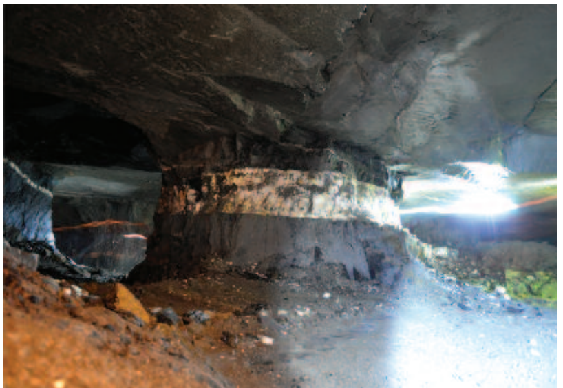
Figure 18 (below): Post-pillar mining in the historic Dolphin mine, Australia. Sand fill by tailings (bottom left) is used as floor for subsequent lifts (drill jumbo is set-up in centre left), making this a combination of cut & fill and room & pillar mining. From HUGHES FE (Ed) [1990]
