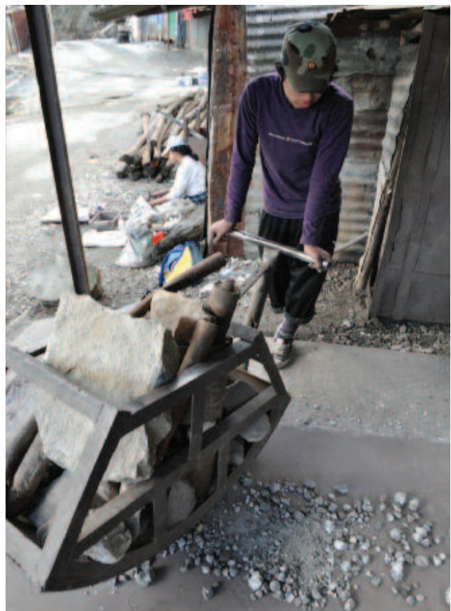
Figure 28: Secondary crushing to grinding in an artisanal operation in Bolivia, using a so-called quimbaleta.
