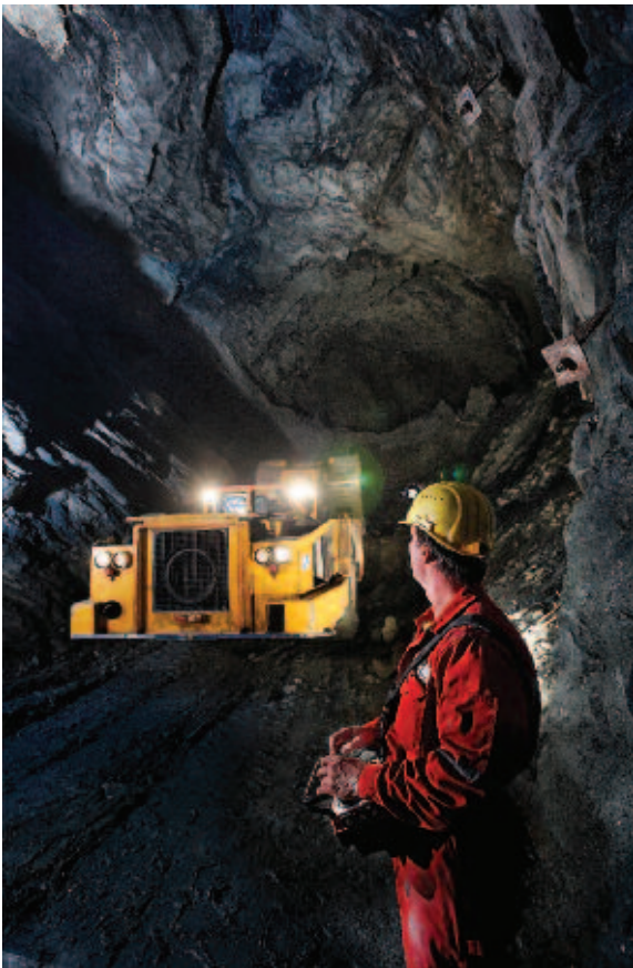
Figures 19 - 20: Sublevel stoping: left mucking of a sublevel stope by remote-controlled scooptram in the Mittersill mine, Austria; above a sketch depicting the set-up of large-scale open stoping using draw-point, from SMITH M (Ed) [2008]
