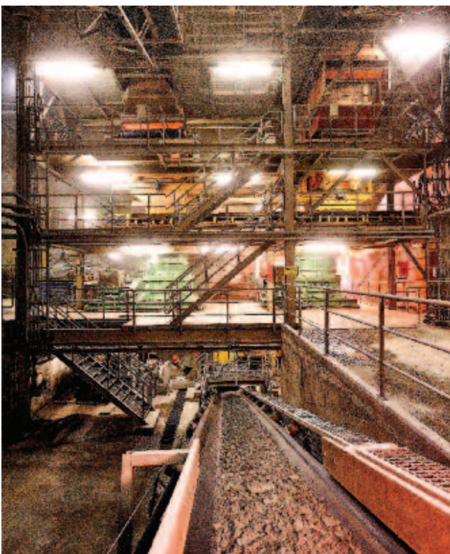
Figures 26 - 27: Primary and secondary crushing in a large underground cavern at Mittersill mine, Austria. Jaw crusher (top) and two cone crushers and sieving plant (bottom).
