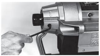
Figure 9 – Loosen the Set Screw
