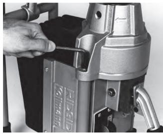
Figure 11 – Remove Socket Head Cap Screws
