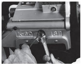
Figure 14 – Tighten Jam Nut
