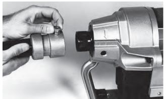
Figure 4 – Rear Guide Hose Attachment
