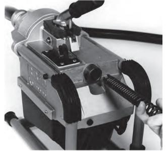
Figure 5 – Inserting Cable Into Front Of Machine
