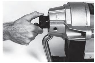
Figure 10 – Jaw Set Adjustment
