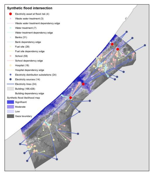
Figure 48: Synthetic flood inundation map for Gaza derived using a DEM for three likelihood bands: significant, moderate and low
