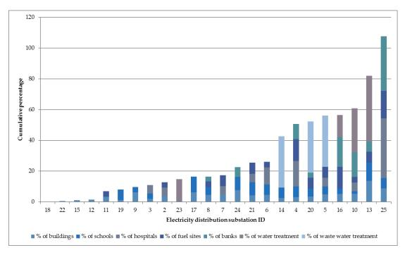
Figure 44: Vulnerability plot showing the magnitude of direct and indirect failure consequences for electricity distribution substation assets (sink assets)
