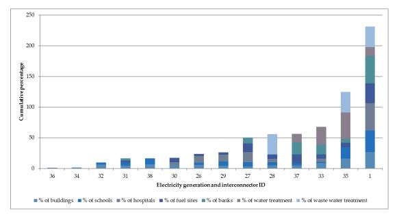
Figure 45: Vulnerability plot showing the magnitude of direct and indirect failure consequences for electricity power stations and interconnector substations (source assets)
