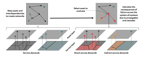
Figure 41: Framework for calculating direct and indirect failure impacts
