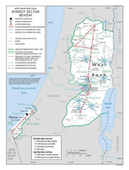
Figure 66: Current and proposed electricity supply system in the West Bank and Gaza (UNISPAL 2007)
