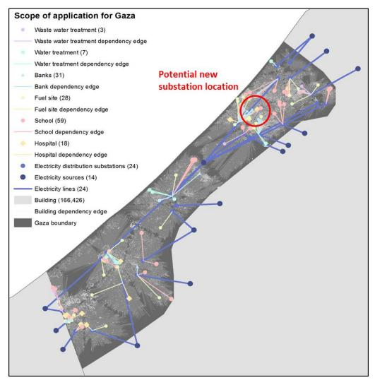
Figure 49: Map highlighting the potential location for a new electricity substation in Gaza city that would distribute the failure risks that currently emerge through the dependencies placed on substations located within the area. The location is also guided through knowledge derived from hazard and previous damage maps
