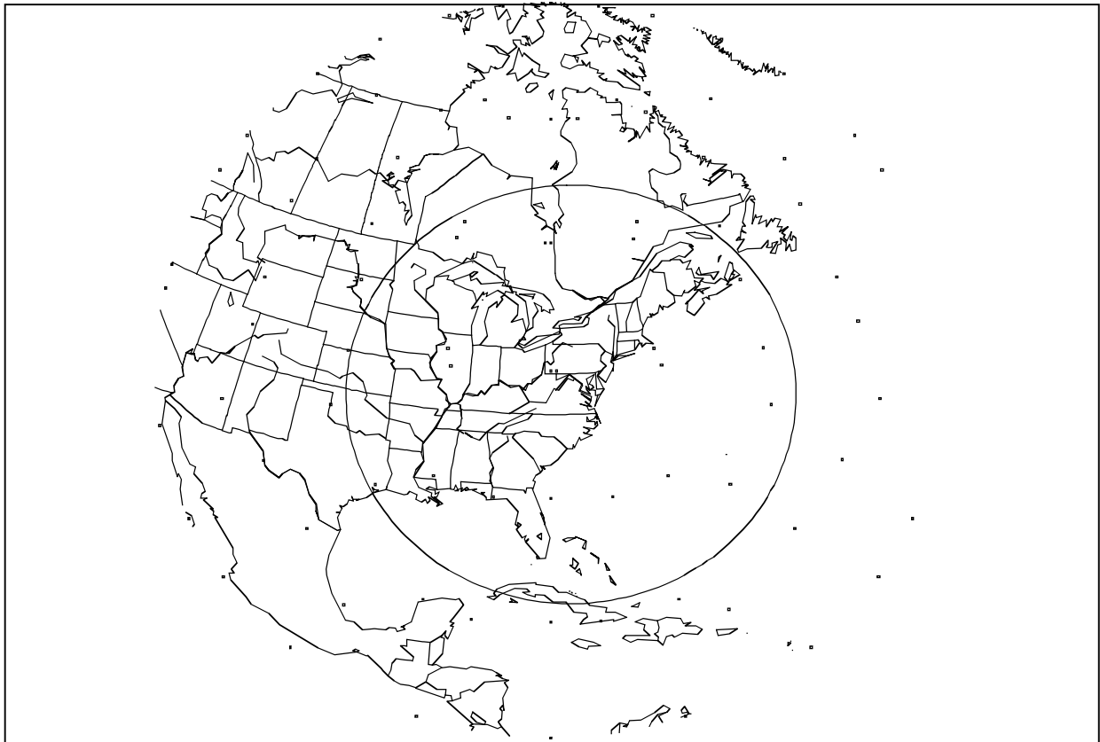
FIGURE 115 Single satellite coverage region, 853 km, 15° elevation angle
