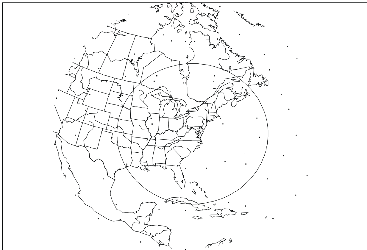
FIGURE 139 Single satellite coverage region, 853 km, 15° elevation angle
