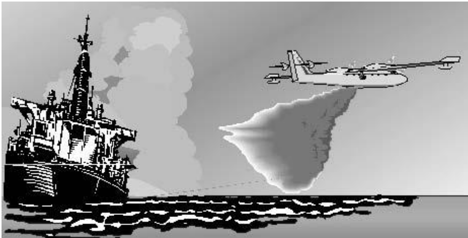
Figure 5 – System for application of dispersant adapted to aircrafts
