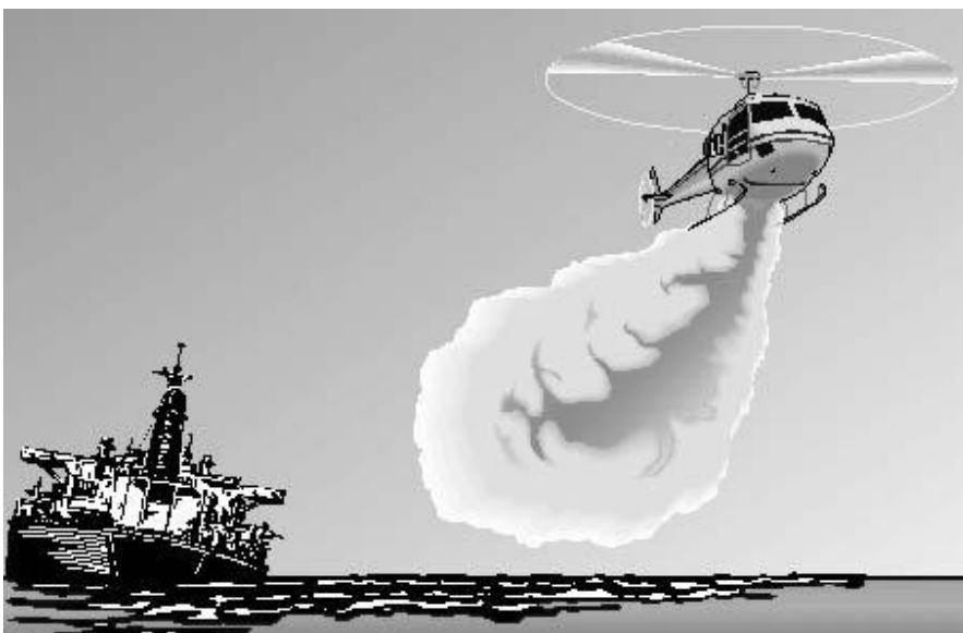
Figure 6 – System for application of dispersant adapted to helicopters
