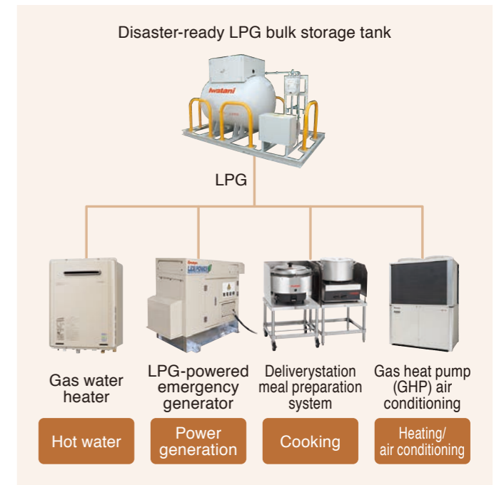
The Iwatani Emergency Energy System
