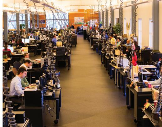
**Wired to work:** One of the most striking aspects of the SEI corporate campus is the network of coiled electrical cables descending from the ceiling. These “pythons,” along with the wheels on every workstation, enable workers to pick up and relocate their mobile desks so new teams can form as the job demands.
