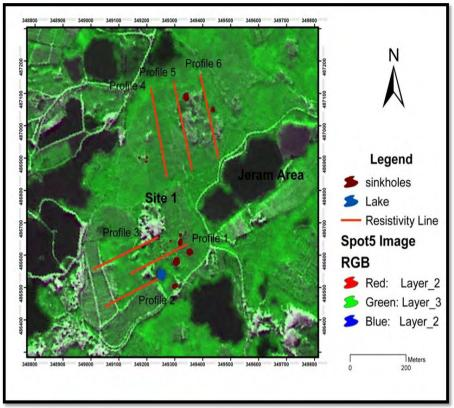
Figure 3: The location of resistivity profile lines
