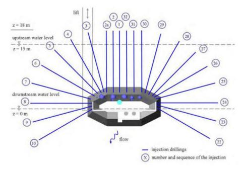
Figure 3. Design of the grouting curtain surrounding the barrage
