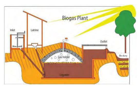
Fig. 12 Typical biogas plant for domestic wastewater
