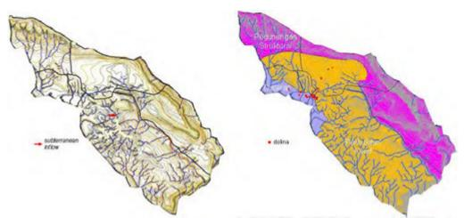
Fig 7 (left). Topographic map of Oksibil. Red arrow indicates subterranean inflow of Oksibil River. Fig 8 (right). Geomorphological map of Oksibil. Red dots indicate location of sinkholes during the survey.
