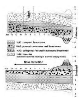
Figure 2. Result of the surface mapping and of the analysis of a vertical drilling in the bottom of the cave [Mutschler and Berner 2005]
