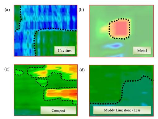
Figure 5. EMP output from several locations: (a) Porous zone, (b) Metal, (c) Compact limestone, (d) Porous limestone
