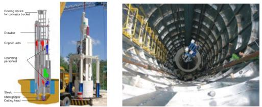
Fig. 7 Application of the vertical drilling machine (left) and view into the developed shaft with a depth of 100 m (left)
