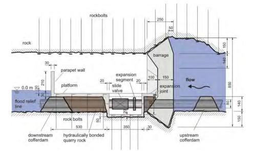
Figure 1. Drawing of the plant (longitudinal section, without components of the hydraulic power plant) with the functional elements cofferdam, flood relief line, barrage and platform with sliding valve chamber [Bohner *et al.* 2009]
