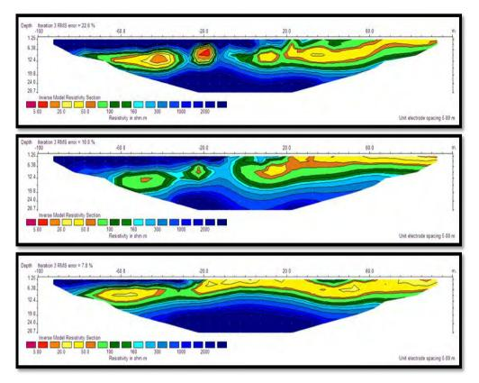
Figure 5: Inverse model of electrical resistivity section for profiles #4, #5 and #6 showing interpreted location of shallow limestone cavities and sinkhole.
