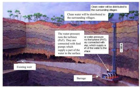
Fig. 5 Basic outline of the underground hydropower plant for water supply (source: Batan / IWG-KIT)
