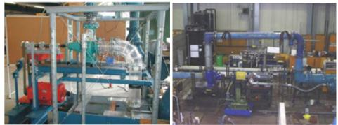
Fig. 3 Test rig to optimize Pump as Turbine (PaT) at the Theodor-Rehbock Water Laboratory, IWG (left) and module 1 (volute casing pump in PaT mode, gearing and multistage centrifugal pump) at the test facility of KSB AG (right)
