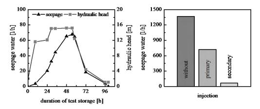
Figure 5. Exemplary graph illustrating the result of a test storage after the secondary injection measure (left) and comparison of seepage water amounts at different stages of the construction process (right)
