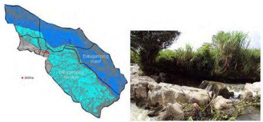
Fig 2 (left). Geological map of Oksibil with distribution of singkholes. Fig 3 (right). A bedded limestones on Oksibil River that tilted N 85° E/10°, camera facing southeast.
