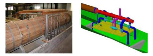
Fig. 13 Experimental investigation of wood-stave pipeline at KIT (left) and illustration of the planned underground hydropower plant in Gua Seropan (right)
