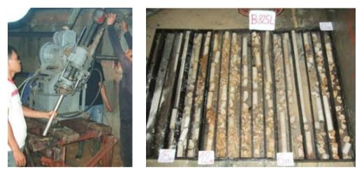
Figure 4. Drilling and injection equipment (left) and drilling cores providing detailed information on the karstification of the rock mass (right)
