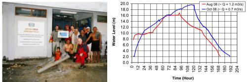
Fig. 12 Successful first storage and operational test in August 2008 (left) and storage curve (right), note: for monitoring purposes, the water level had constantly been held at several heights through partial opening of the controlling valves
