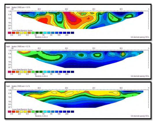
Figure 4: Inverse model of electrical resistivity section for profiles #3, #1 and #2 showing interpreted location of shallow limestone cavities and sinkhole.
