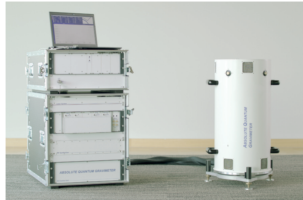
AQG is composed of the sensor head (right side of the image) where the gravity measurement is performed, and the control unit (left side of the image)
