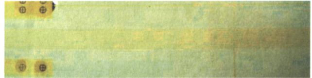
Figure 7: Ion exchanged waveguides after diffusion mask removal with positioning marks (1x8 cm)
