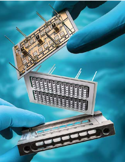
Half bridge module for a directly cooled AC/DC converter for a Formula 1 car
