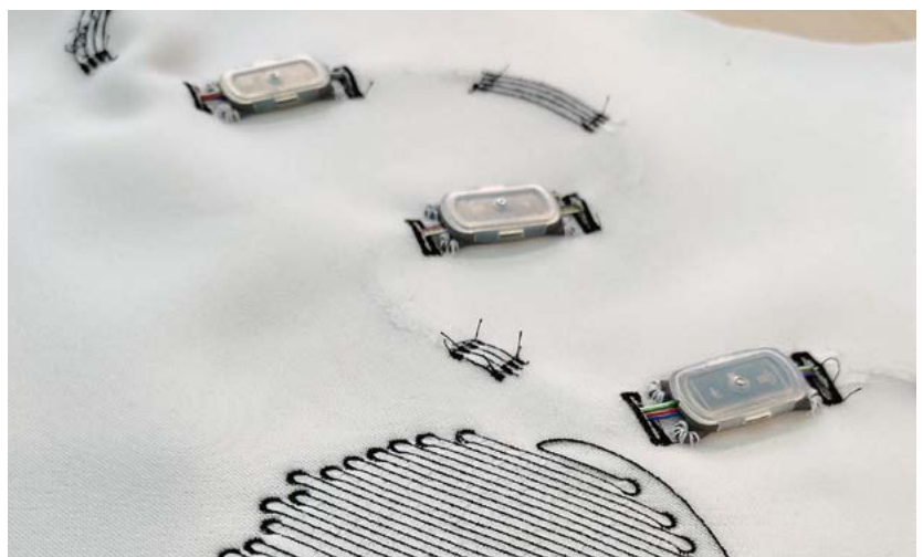
bottom: Current case design for a Bionic RoboSkin sensor skin mounted by Fraunhofer IZM's project partner TITV
