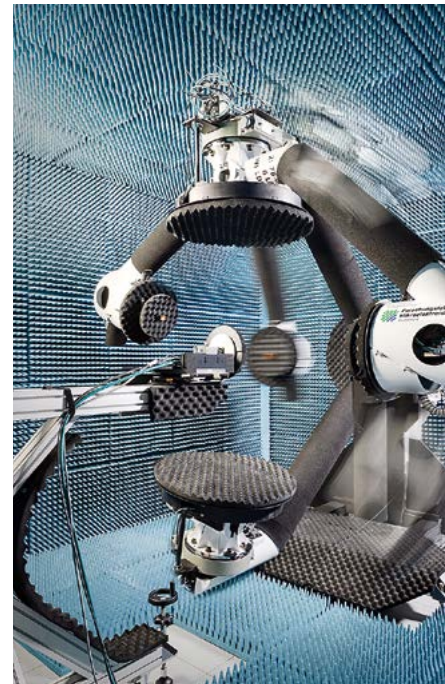
Automated antenna measuring station for near and far-field measurements at up to 325 GHz
