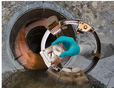
left: Autonomous sensor system for monitoring environmental conditions in sewers
