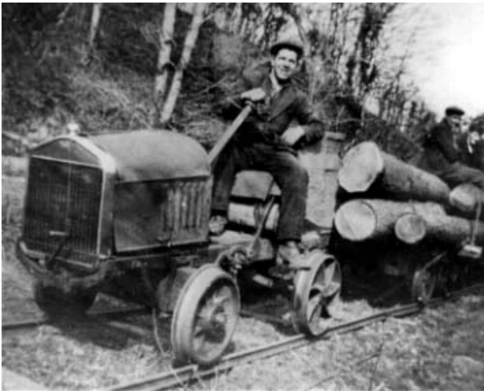
A Ford Model T engine powers this locomotive on the light railway constructed to ferry timber at a site on Arran in the 1930s.
