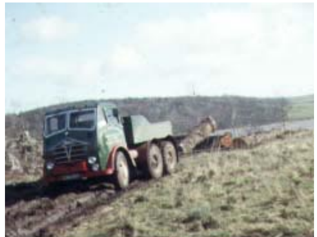
This six-wheel Foden, in operation at St Mary's Isle in Kirkcudbrightshire around 1960, was converted for harvesting use from an ex-RAF lorry by James Jones's engineering workshop. The lorry was cut down, the cab rebuilt and a winch fitted. (Courtesy of Airlie Bruce-Jones.)
