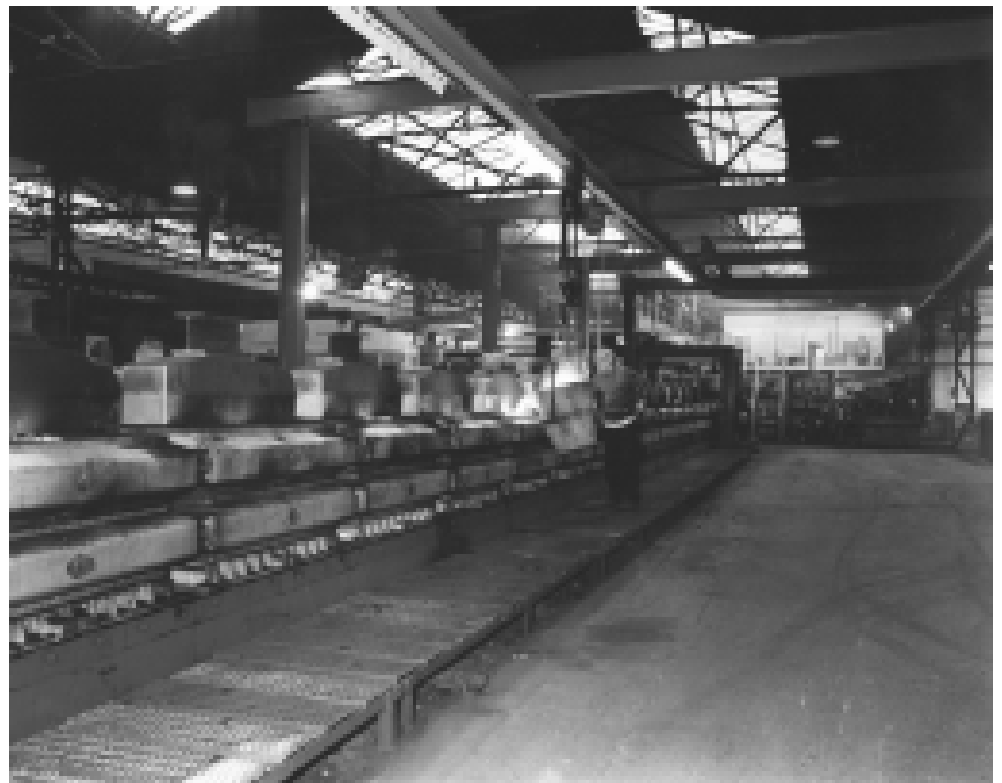
Moulds being created (brake drums for Albion Motors in Glasgow); and hot metal being poured by hand into the moulds before the advent of automatic moulding in 1982.
