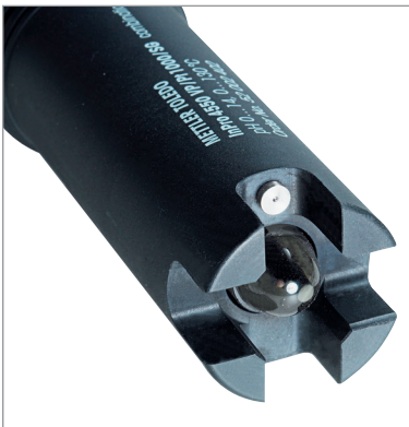
Slotted tip protects the pH glass membrane
