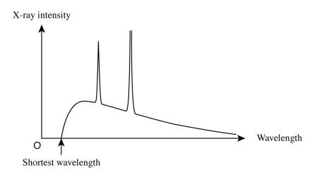
Q1 If we increase the kinetic energy of the electrons by increasing the accelerating voltage, what would happen to the wavelength at the sharp peaks, and the shortest wavelength? 19 From (1)-(7) below choose the correct combination.
