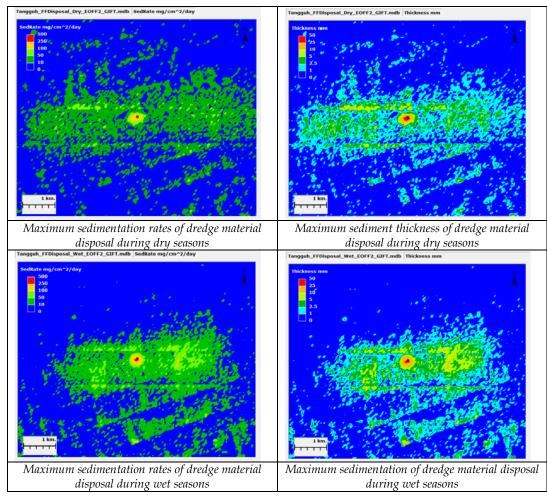
Figure III-71 Modeling Results of Maximum Sedimentation Rates and Maximum Sedimentation Thickness during Dry Seasons and Wet seasons
