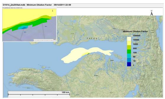
Figure III-54 Contour of Minimum Dilution Factor at LNG 2 Jetty in the Dry Season
