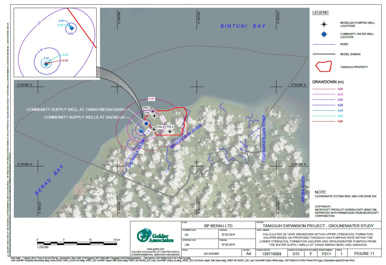
Figure III-41 Modeling of Water Table for 29 Year in the Upper Steenkool Formation Aquifer based on Pumping of Community Wells and Proposed Groundwater at the Tangguh LNG
