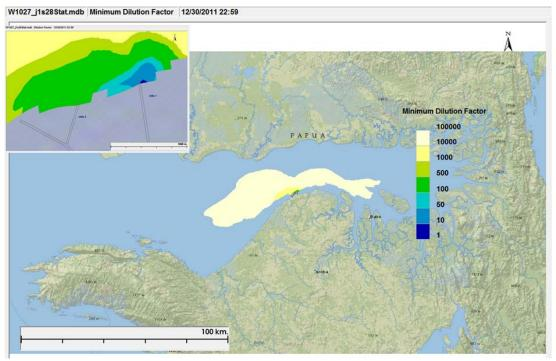
Figure III-53 Contour of Minimum Dilution Factor at LNG 1 Jetty in the Wet Season
