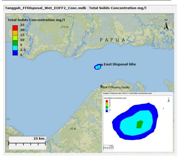
Figure III-65 Spread of Maximum Increased TSS during the Disposal of Dredge material in the East Disposal during Wet seasons
