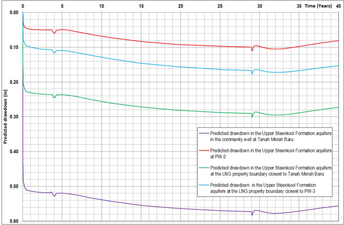
Figure III-42 Predicted Drawdown and Rebound of Water Level in Upper Steenkool Formation Aquifer at PW-2, Community Well at Tanah Merah Baru, at the Boundary Area of the Tangguh LNG nearest to PW-3 and the Boundary Area of the Tangguh nearest to Tanah Merah Baru Village
