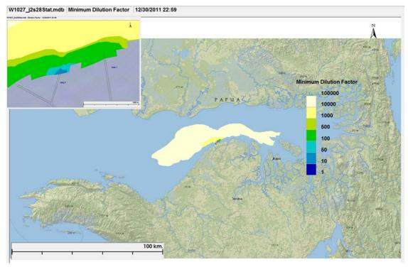
Figure III-55 Contour of Minimum Dilution Factor at LNG 2 Jetty in the Rainy Season
