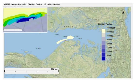
Figure III-27 Minimum Dilution Factor Contour Plot of the Combined Hydrotest Water and Comingled Wastewater at the LNG Jetty 2 during the Wet season
