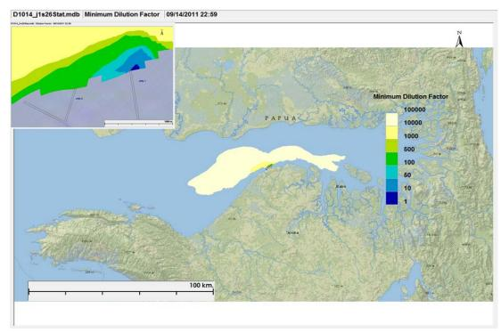
Figure III-52 Contour of Minimum Dilution Factor at LNG 1 Jetty in the Dry Season
