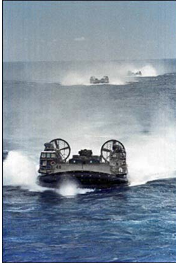
Landing craft, air cushion vehicles provide the over-the-horizon heavy lift capability for the landing force.
