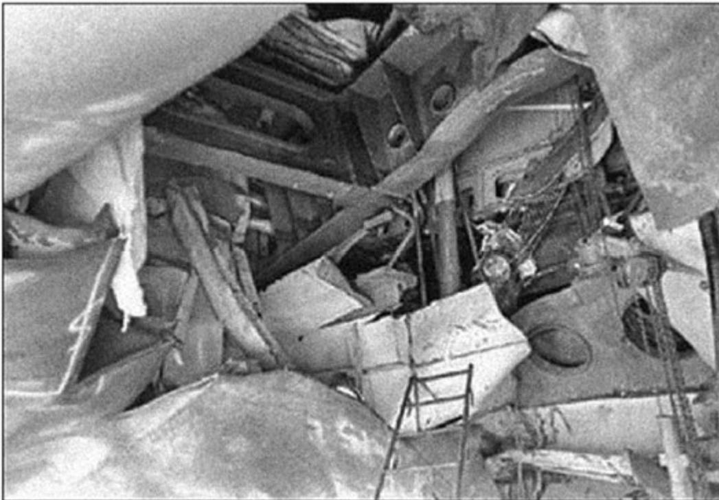
Estimated to cost about $1,500, an unsophisticated contact mine that was based on a 1908 Russian design caused some $96 million in damage in 1987 to the frigate United States Ship Samuel B. Roberts (FFG-58), shown above with damage to the hull as seen from dry dock, almost causing the ship to sink.
