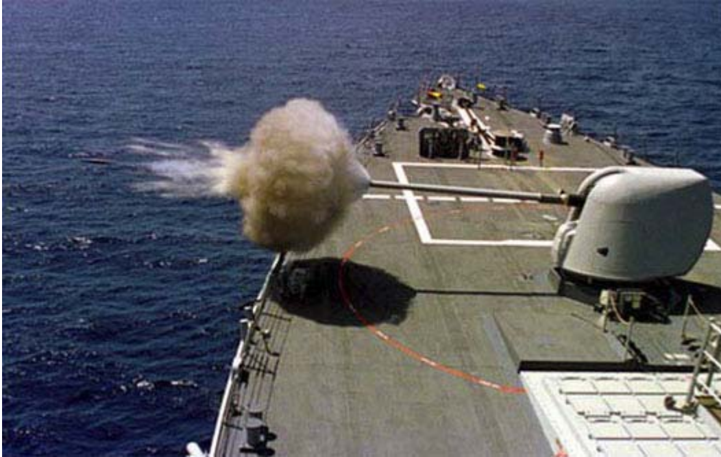
Arleigh Burke-class guided missile destroyers are equipped with a 5-inch (127-millimeter) gun.
