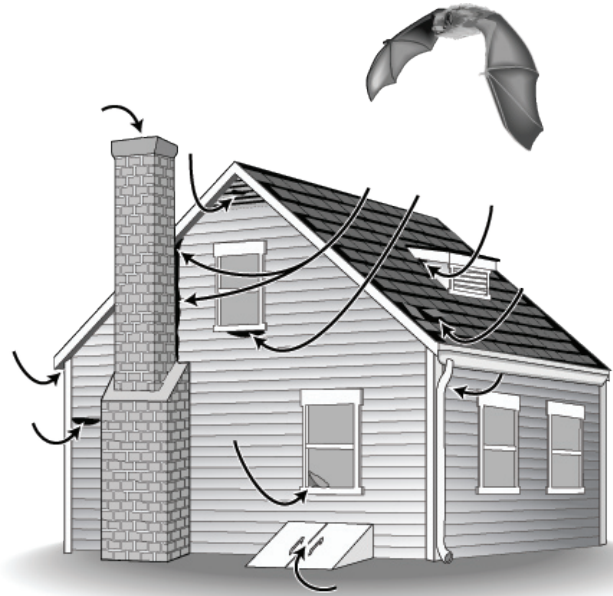
Figure 1. Bats may gain access to a structure through a variety of entry points in their attempt to roost.
