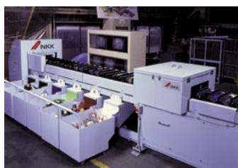
Wastes sorting and recycling system
