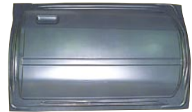
Example of applications of HITEN (door panel experimentally produced by the 1200-ton press)
