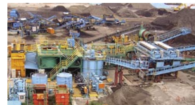
Water washing & classifying soil remediation system
