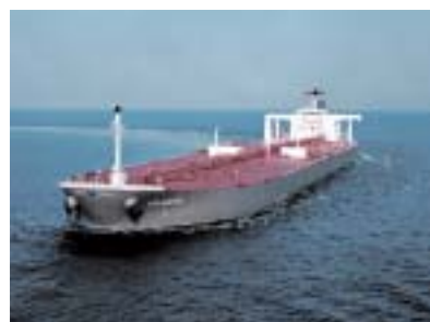
Tanker constructed using TMCP high strength steel plates
