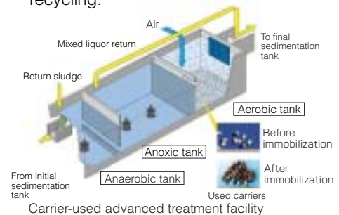
Carrier-used advanced treatment facility
