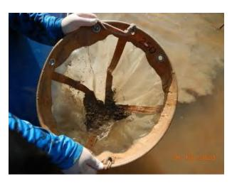
Figure 434 – The washing of the sediments on a sieve with an aperture of 250  $\mu$ m.
