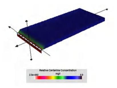
$Figure \ 11-Simulation \ of \ the \ color \ dispersion \ plume \ in \ 3 \ dimensions.$
