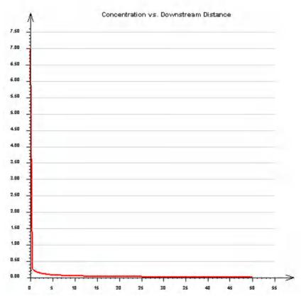
Figure 18 – Graphic of nitrogen concentration (mg/L) X distance (m).
