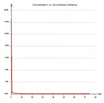
Figure 10 - Graphic of BOD concentration (mg/L) X distance (m).
