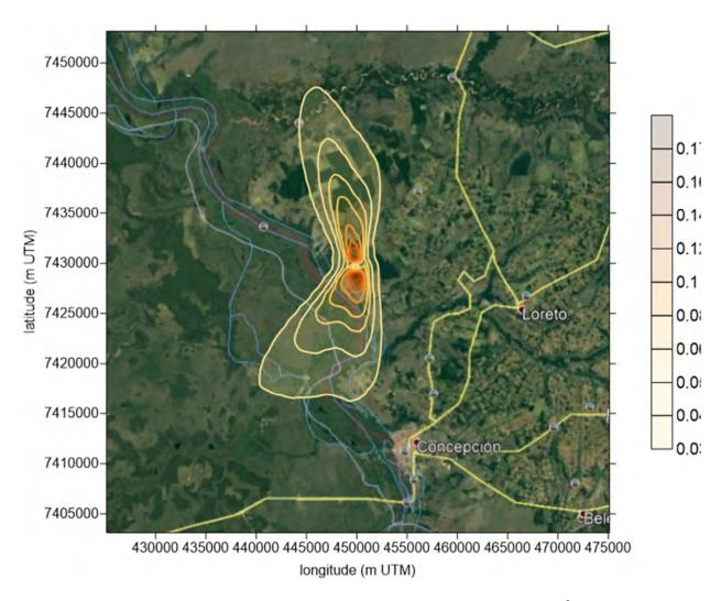
**Figure 24** – Maximum annual average concentration for  $PM_{10}$  (scale in  $\mu g.m^{-3}$ ). Maximum peak concentration of 0.17252  $\mu g.m^{-3}$  at position 7428625 S and 449875 O (m UTM).
