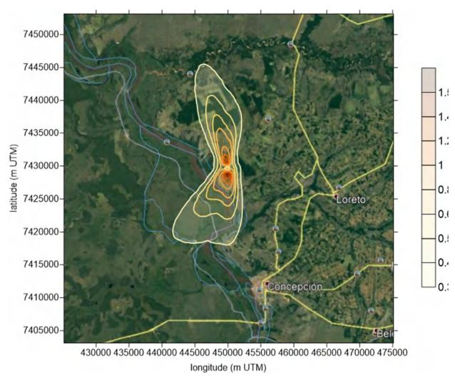
**Figure 22** – Maximum annual average  $NO_2$  concentration (scale in  $\mu g.m^{-3}$ ). Maximum peak concentration of 1.57742  $\mu g.m^{-3}$  at position 7428625 S and 449875 O (m UTM).
