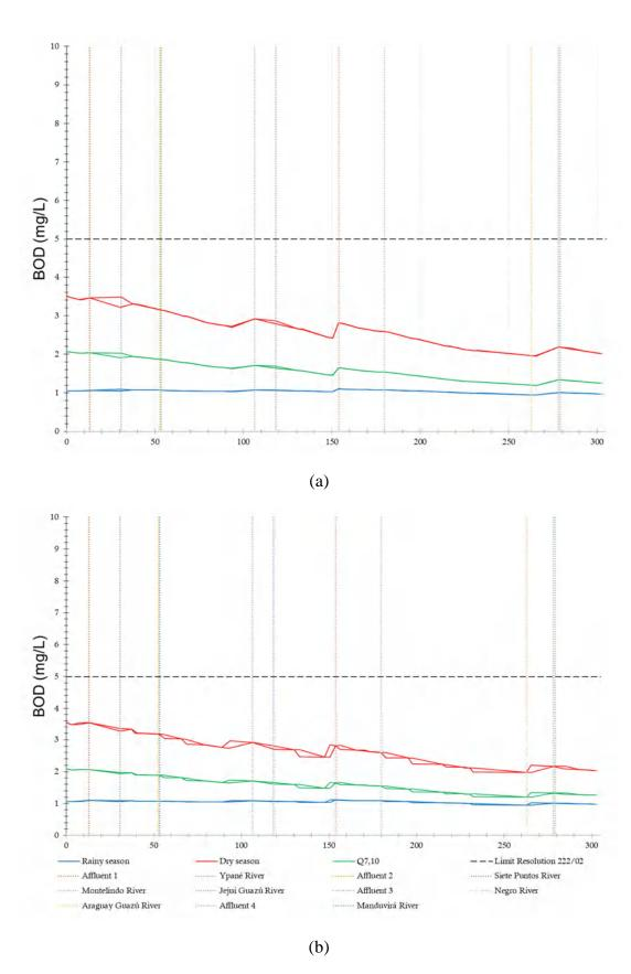
Figure 15 - Longitudinal profiles of BOD: (a) Current situation; (b) Future situation after the treated effluent discharge.
