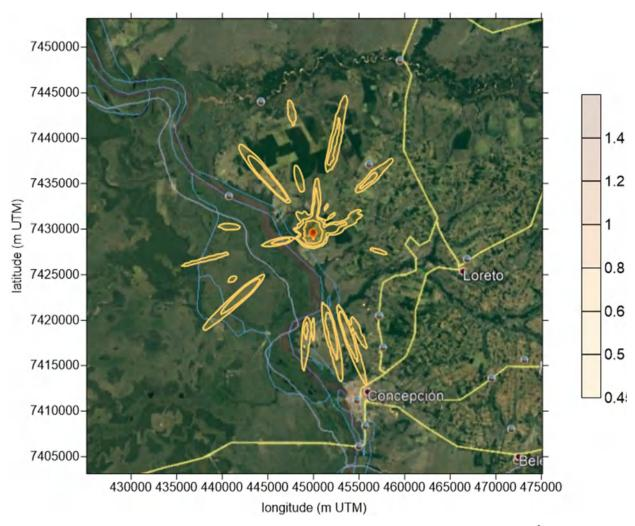
**Figure 19** – Maximum average concentration of 1 hour for TRS (scale in  $\mu g.m^{-3}$ ). Maximum peak concentration of 1,49240  $\mu g.m^{-3}$  at position 7429875 S and 449875 O (m UTM) on 02/24/2018 at 12 h.
