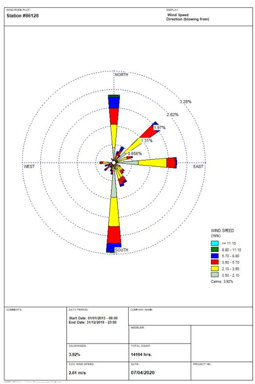
Figure 36 – Wind rose observed at Pozo Colorado station
