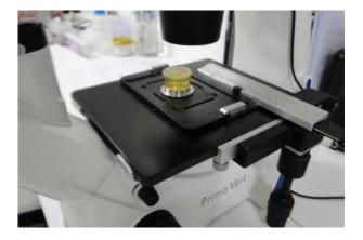
Figure 431 – Utermöhl camera sample.
