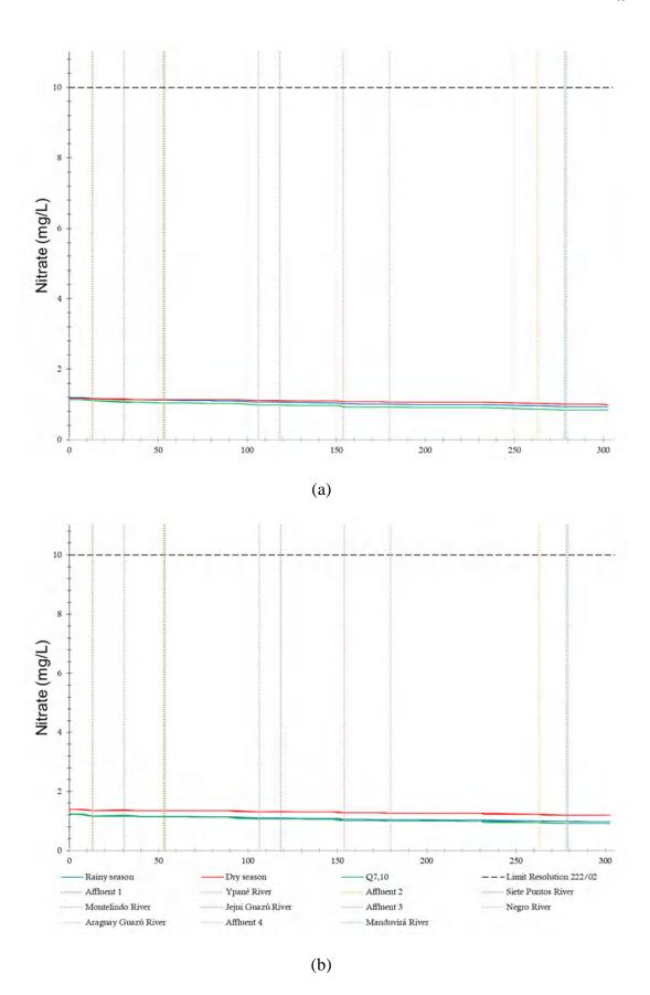
Figure 17 - Longitudinal profiles of nitrate: (a) Current situation; (b) Future situation after the treated effluent discharge.
