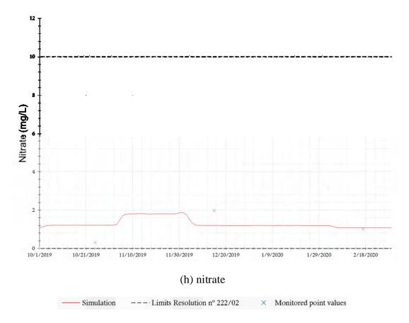
Figure 9 - Fit between simulated profiles and monitored data in WQS-2. Author (2021).
