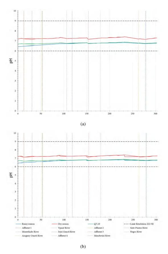
Figure 12 - Longitudinal profiles of pH: (a) Current situation; (b) Future situation after the treated effluent discharge.
