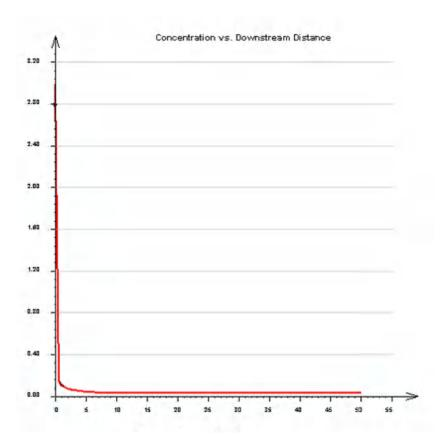
Figure 24 – Graphic of AOX concentration (mg/L) X distance (m).
