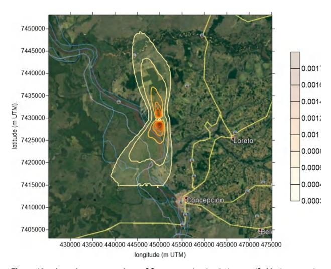
**Figure 18** – Annual average maximum CO concentration (scale in mg.m<sup>-3</sup>). Maximum peak concentration of 0.00174 mg.m<sup>-3</sup> at position 7428625 S and 449875 O (m UTM).
