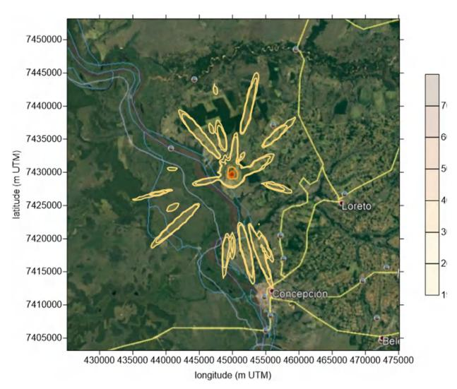
**Figure 21** – Maximum average concentration of 1 hour for  $NO_2$  (scale in  $\mu g.m^{-3}$ ). Maximum peak concentration of 74.81947  $\mu g.m^{-3}$  at position 7429875 S and 449875 O (m UTM) on 02/24/2018 at 12 h.
