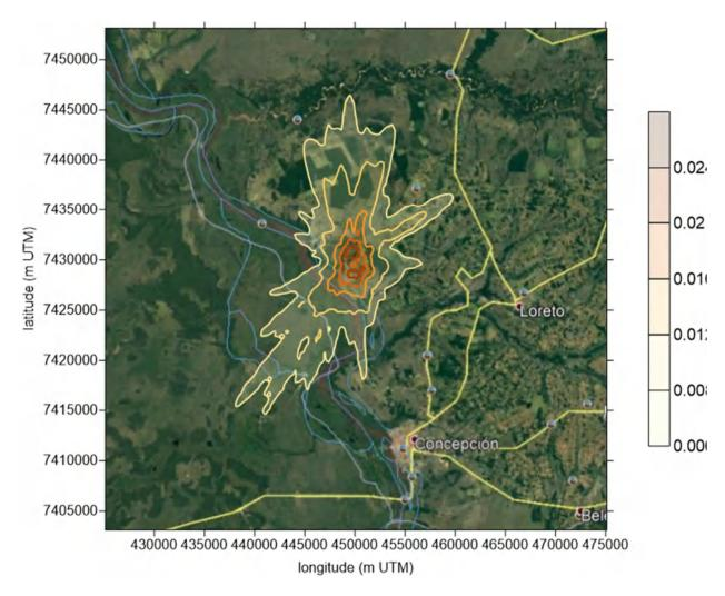
**Figure 17** – Maximum average concentration of 8 hours for CO (scale in  $mg.m^{-3}$ ). Maximum peak concentration of 0.02490  $mg.m^{-3}$  at position 7430625 S and 449875 O (m UTM) on 04/02/2019 at 4 p.m.
