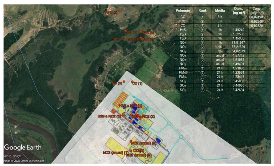
Figure 27 – Location of the highest concentrations around the pulp mill.
