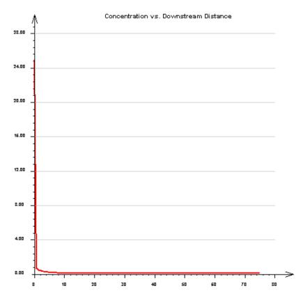
Figure 8 – Graphic of BOD concentration (mg/L) X distance (m).
