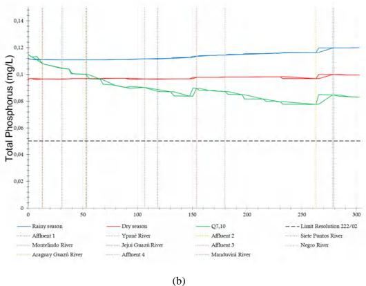
Figure 18 – Longitudinal profiles of total phosphorus: (a) Current situation; (b) Future situation after the treated effluent discharge.
