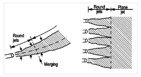
Figure 5 – Discharge of effluent by diffusers.
