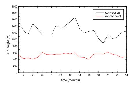
**Figure 16** – Temporal evolution (monthly average) of the height of the CLA calculated by AERMET for the pulp mill site in the period between 01/01/2018 and 01/01/2020.
