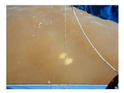
Figure 425 – Measuring transparency with the Secchi disk.
