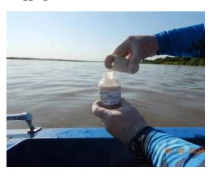
$\begin{array}{lll} Figure & 430 & - & Phytoplankton & sample \\ conditioning. & & & \end{array}$
