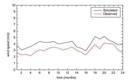
**Figure 11** – Comparison between the average monthly wind speed simulated by the WRF and that observed at the Teniente Coronel Carmelo Peralta airport station (USAF: 861340 / ICAO: SGCO) from 01/01/2018 to 12/31/2019.
