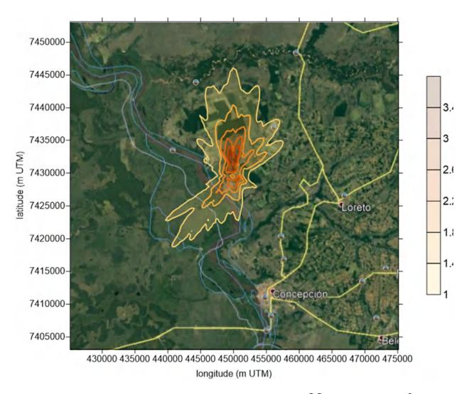
**Figure 25** – Maximum 24-hour average concentration for  $SO_2$  (scale in  $\mu g.m^{-3}$ ). Peak concentration peak of 3.45833  $\mu g.m^{-3}$  at position 7432125 S e 449625 O (m UTM) on 08/13/2019.
