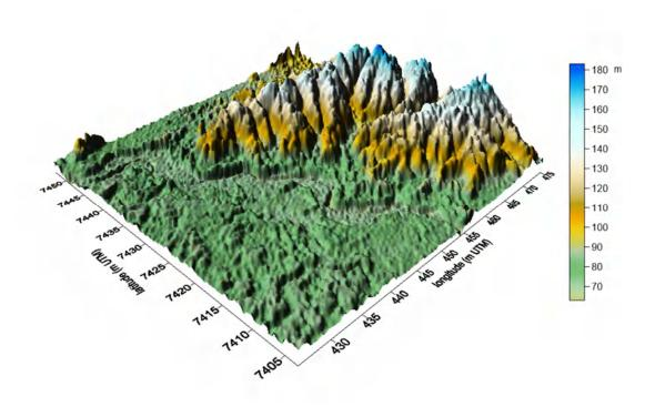
**Figure 1** –Three-dimensional orographic map of the study area (2,500 km²). Source: Generated with SRTM-NASA data ("Shuttle Radar Topography Mission - NASA") with 90 m of definition.
