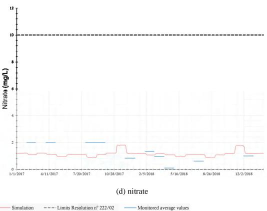
Figure 11 - Fit between simulated profiles and monitored data in WQS-4. Author (2021).
