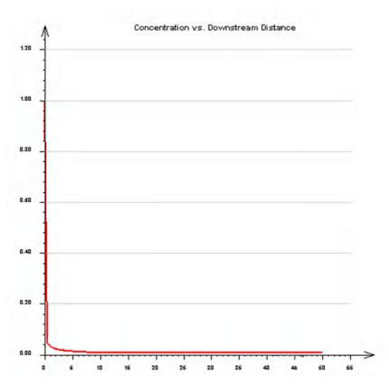
Figure 20 – Graphic of phosphorus concentration (mg/L) X distance (m).
