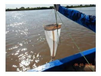
Figure 427 – The 20  $\mu m$  network for qualitative sampling.
