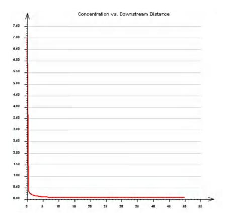
Figure 16 – Graphic of nitrogen concentration (mg/L) X distance (m).
