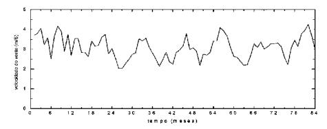
Figure 35 – Average wind speed at station Pozo Colorado
