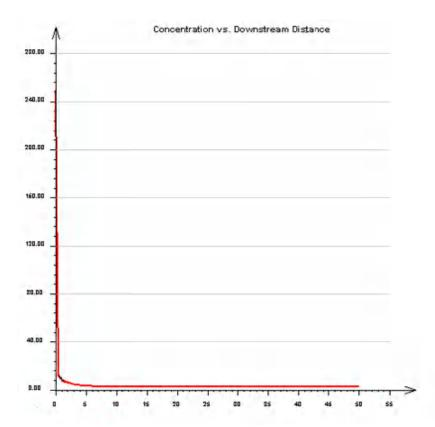
Figure 12 – Graphic of color concentration (mg/L) X distance (m).
