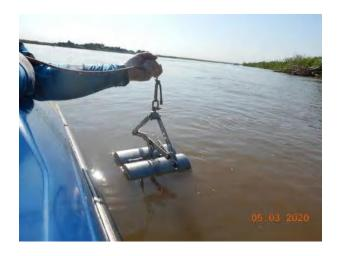
Figure 433 – The Petersen dredger used to collect benthic invertebrates.
