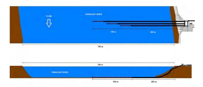
Figure 15 – Illustration of the discharge system
