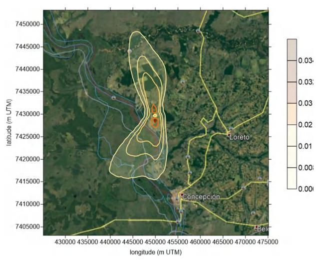
**Figure 20** – Maximum annual average concentration for TRS (scale in  $\mu g.m^{-3}$ ). Maximum peak concentration of 0.03424  $\mu g.m^{-3}$  at position 7428625 S and 449875 O (m UTM).
