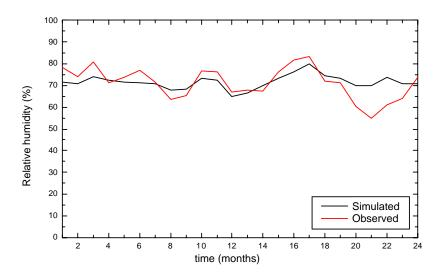
**Figure 10** – Comparison between the monthly relative humidity simulated by the WRF and that observed at the Teniente Coronel Carmelo Peralta airport station (USAF: 861340 / ICAO: SGCO) from 01/01/2018 to 12/31/2019.
