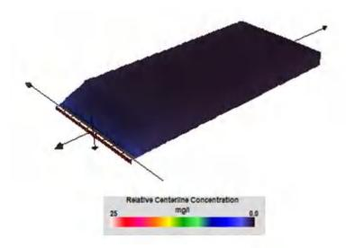
Figure 9 – Simulation of the BOD dispersion plume in 3 dimensions.
