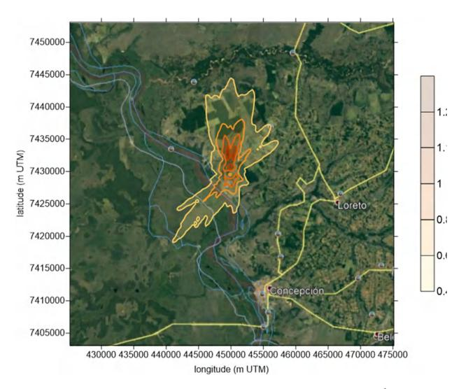
**Figure 23** – 24-hour average maximum concentration for  $PM_{10}$  (scale in  $\mu g.m^{-3}$ ). Maximum peak concentration of 1.23890  $\mu g.m^{-3}$  at position 7432125 S and 450 125 O (m UTM) on 08/02/2019.
