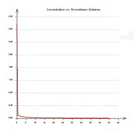
Figure 26 – Graphic of AOX concentration (mg/L) X distance (m).
