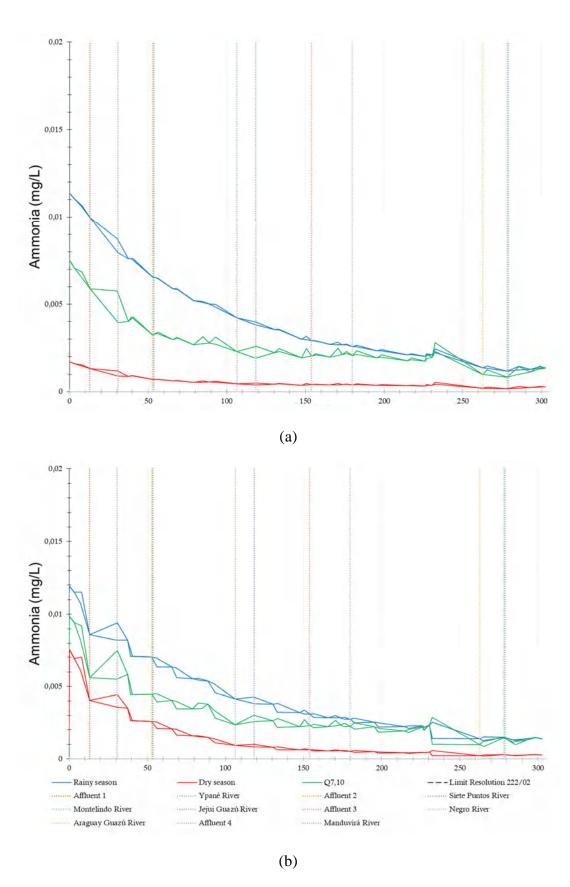
Figure 16 - Longitudinal profiles of ammonia: (a) Current situation; (b) Future situation after the treated effluent discharge.
