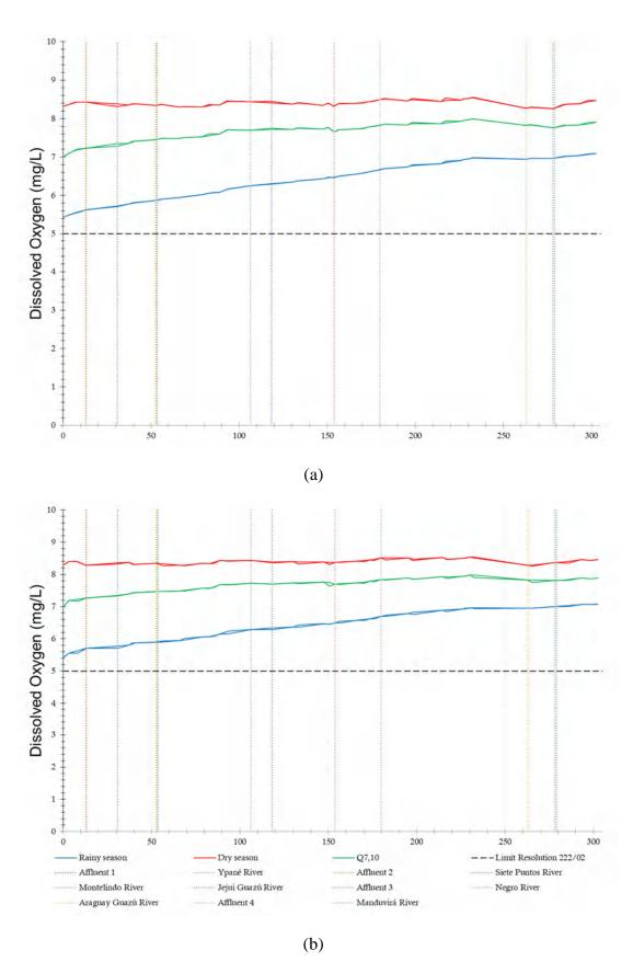
Figure 14 - Longitudinal profiles of dissolved oxygen: (a) Current situation; (b) Future situation after the treated effluent discharge.
