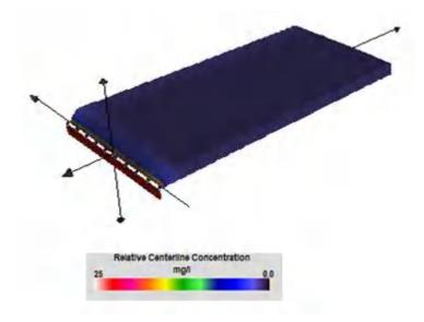
Figure 7 – Simulation of the BOD dispersion plume in 3 dimensions.
