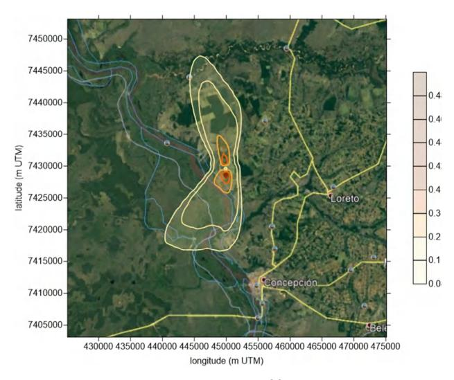
**Figure 26** – Maximum annual average concentration for  $SO_2$  (scale in  $\mu g.m^{-3}$ ). Maximum peak concentration of 0.47616  $\mu g.m^{-3}$  at position 7428625 S and 449875 O (m UTM).
