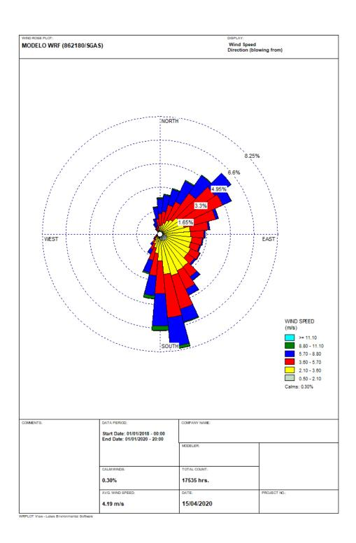
**Figure 15** – Wind rose generated from data simulated by the WRF model at the coordinates of the Silvio Pettirossi International Airport station (USAF: 862180 / ICAO: SGAS) from 01/01/2018 to 01/01/2020.
