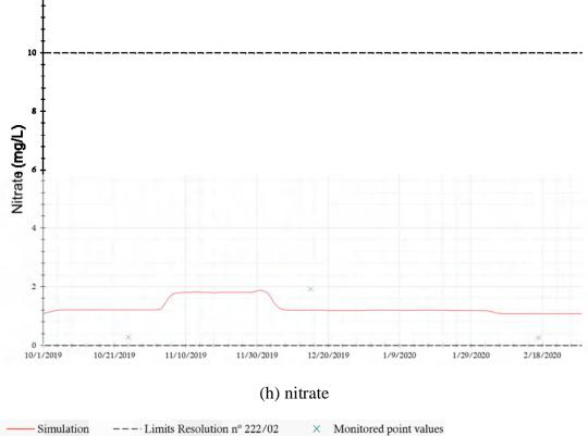
Figure 10 - Fit between simulated profiles and monitored data in WQS-3. Author (2021).
