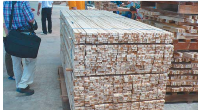
Fig.3. Finger jointed teak lumber at Nong Khai ANP Import and Export Co.Ltd., Nong Khai Province
