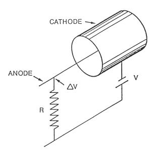
Two electrode, gas filled chamber
