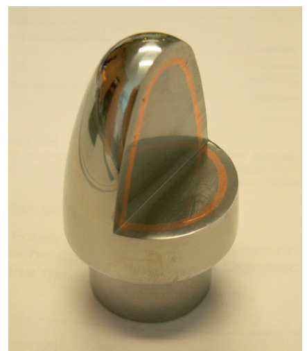
Fig. 3: Part made from three different materials
