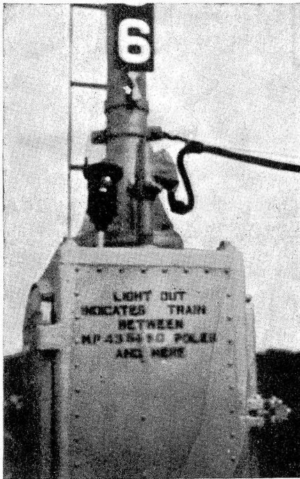
Lamp-type train-approach indicator on color-light signal territory
